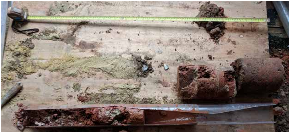
Plate 13: Complete core from WS106 showing brick obstruction. Right to left.
