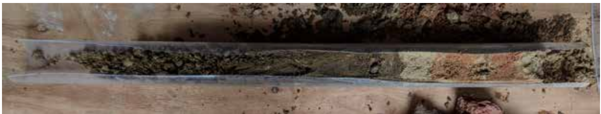
Plate 11: The core from 1.00-2.00m BGL (left to right) from WS104. 0.00-1.00m was concrete and brick which was cored and was unphotographable.
