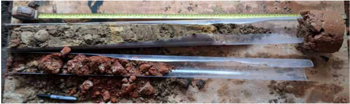
Plate 12: Complete cores from WS105 showing brick obstruction. Top to bottom, right to left.
