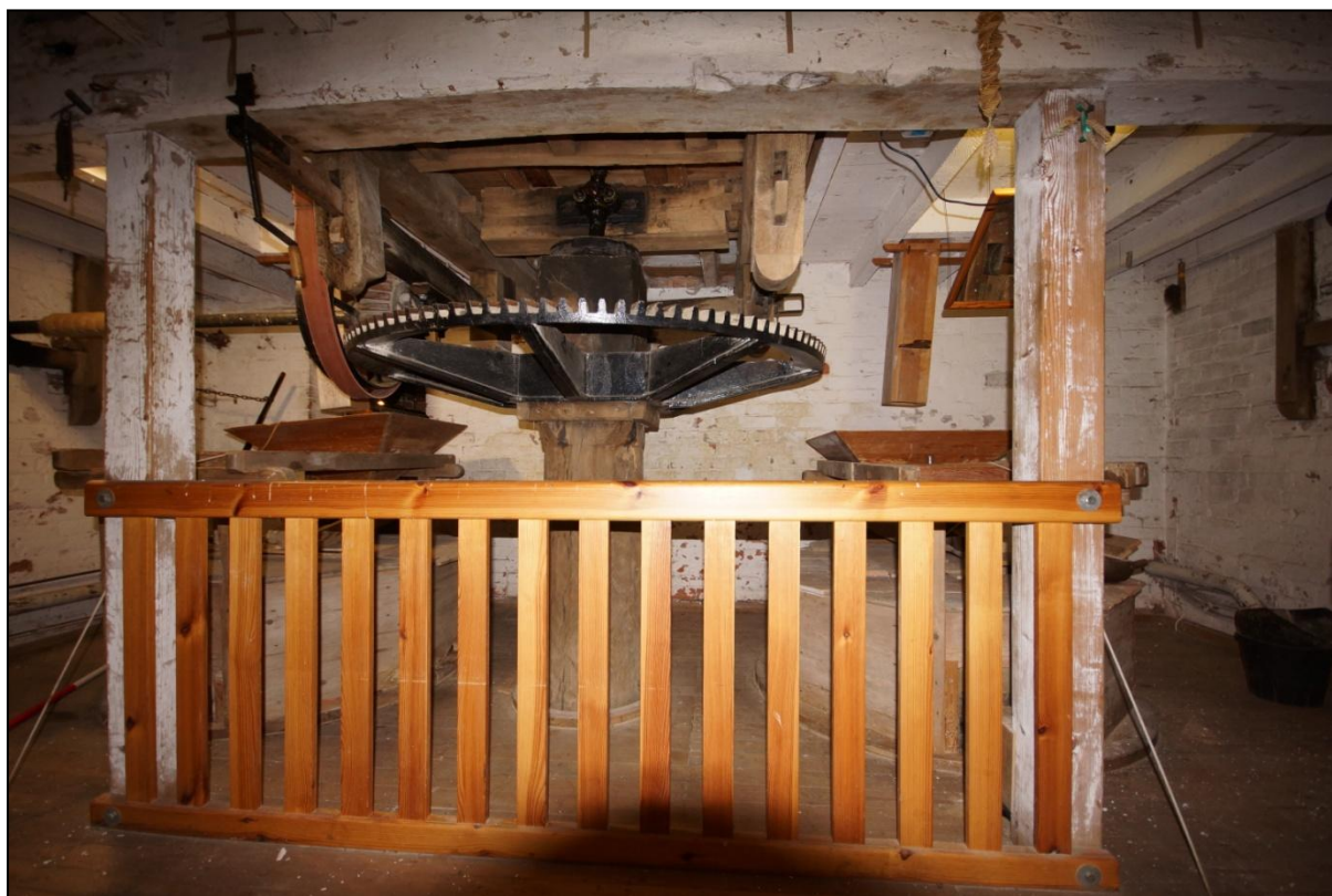
Plate 64: The crown wheel of the first floor of Building 08, viewed looking west.
