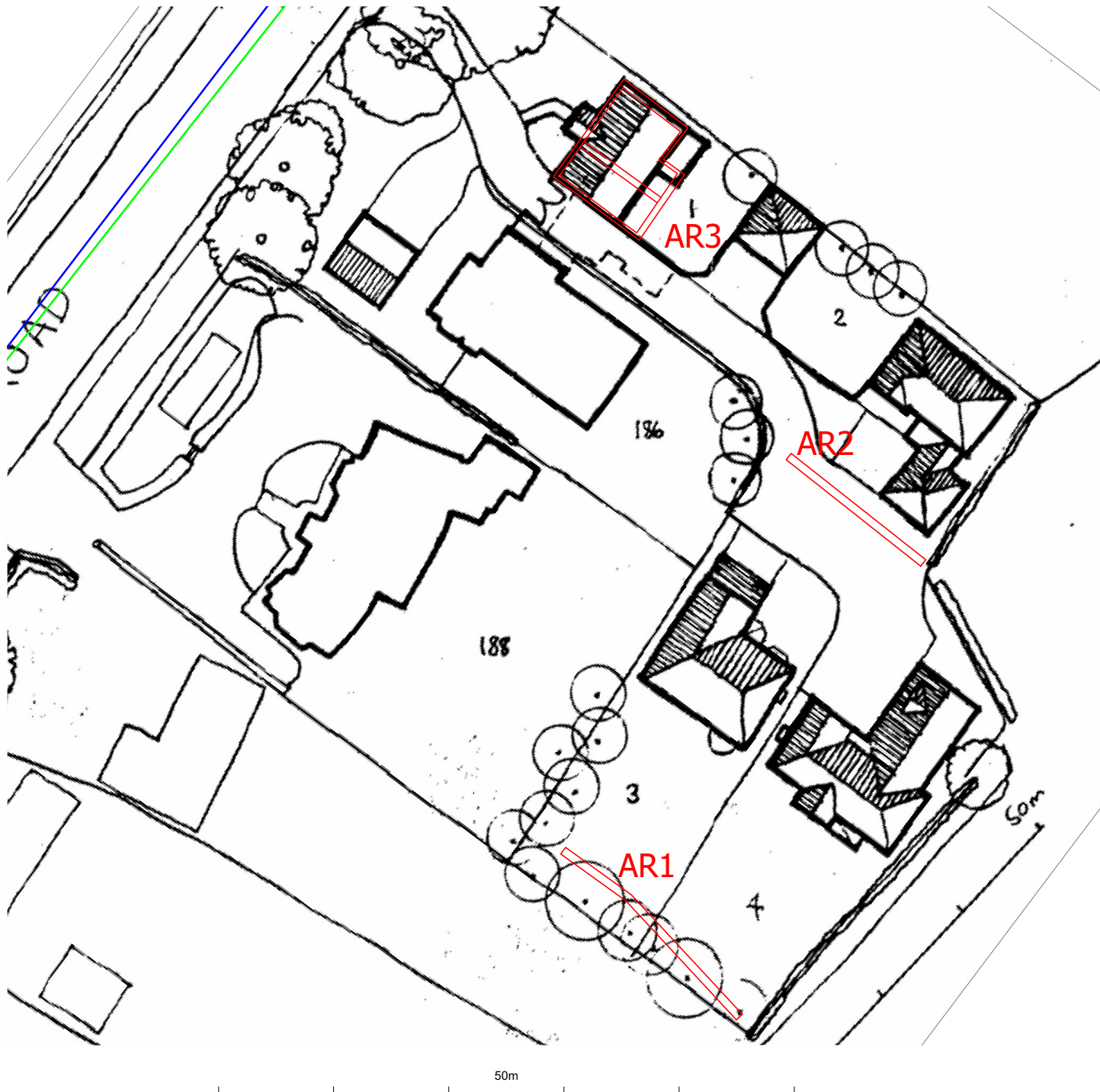
Fig. 3: trenches inspected (red) and existing site layout with proposed new dwellings 1-4, showing actual course of A38 (blue) and greatest length of Roman road which can be projected as a straight course between apparent surviving stretches (green; dot-dashed)
