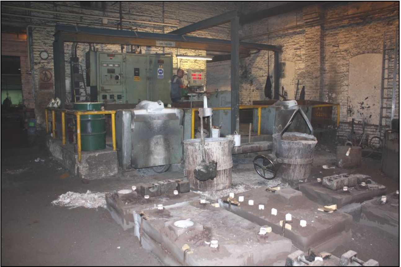
Plate 18: The Canlin Castings Ltd site at Langley Mill: present-day furnaces at the north end of the large castings floor in Building 7C.
