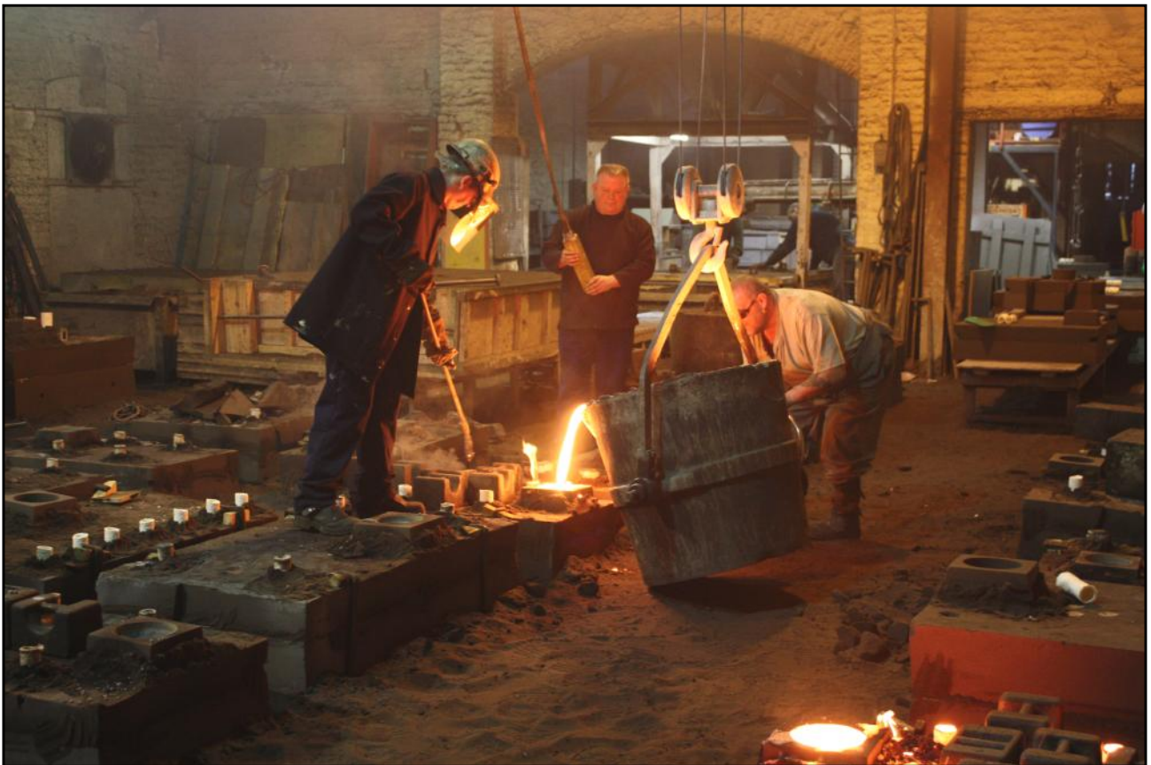
Plate 19: The Canlin Castings Ltd site at Langley Mill: molten iron being poured into moulds in the large castings floor in Building 7C.
