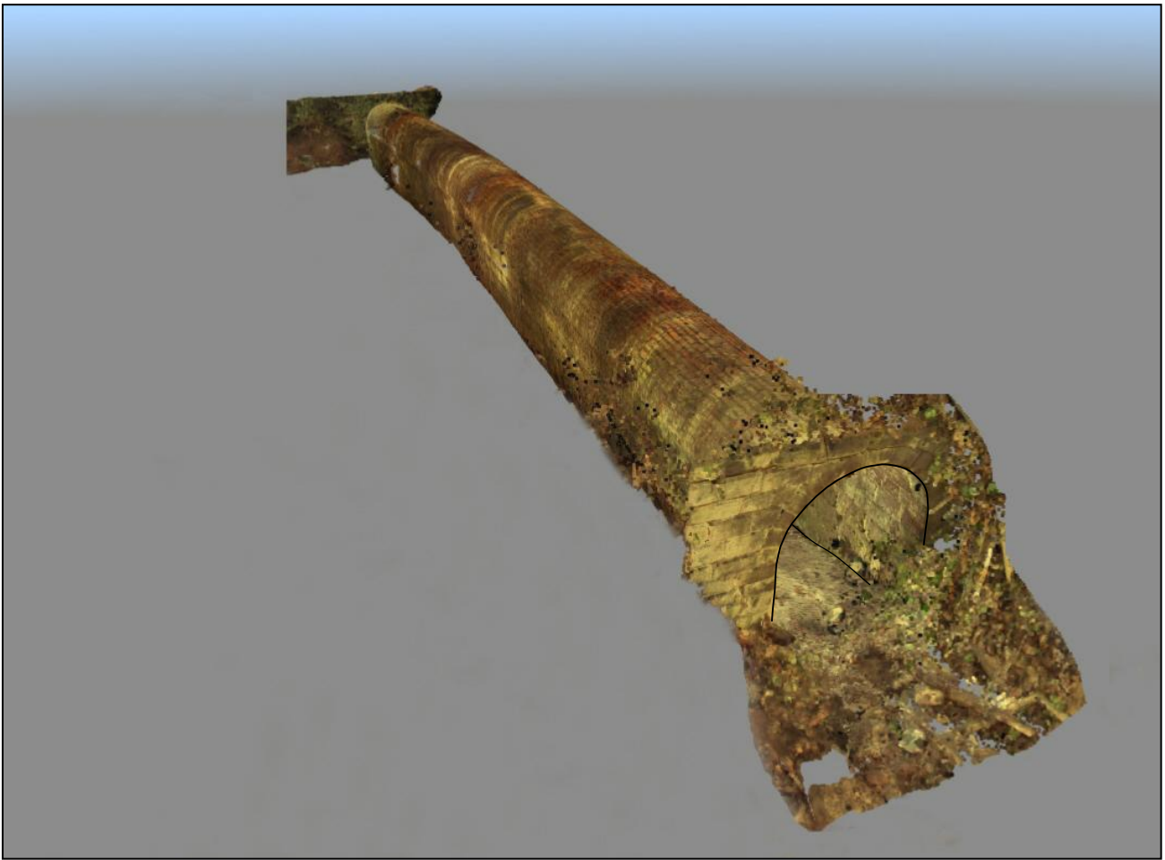
Figure 11: Perspective view of the south end of the Long Tunnel derived from a 3D laser scanner survey at Loner's Lair, Duffield Bank, Derbyshire.
