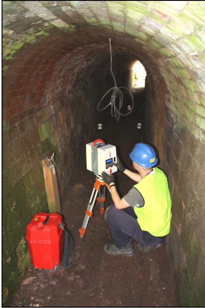
Plate 13: Laser scanner being operated within the Long Tunnel at Duffield Bank.
