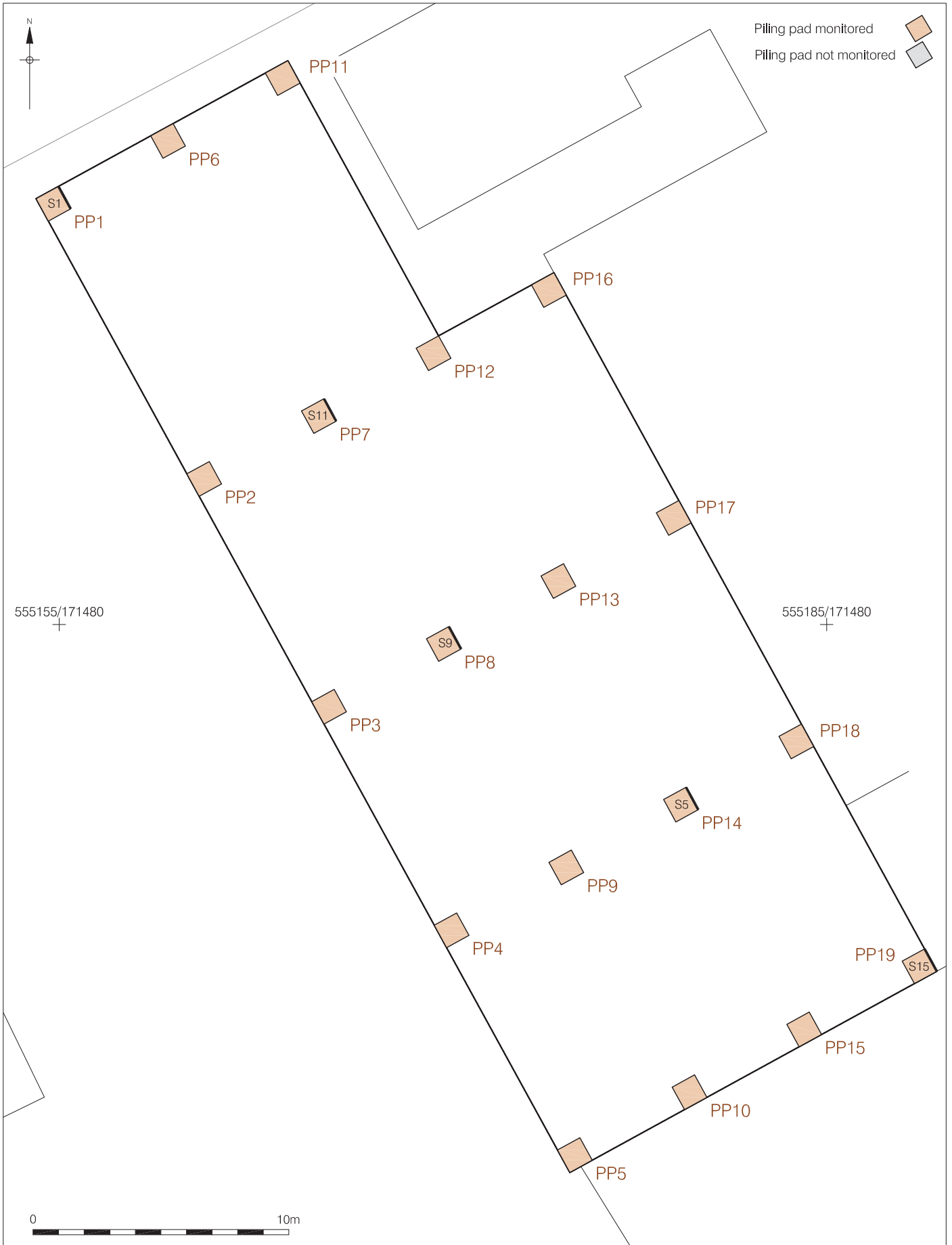
Figure 4 Piling locations for New Covers 1:200 at A4
