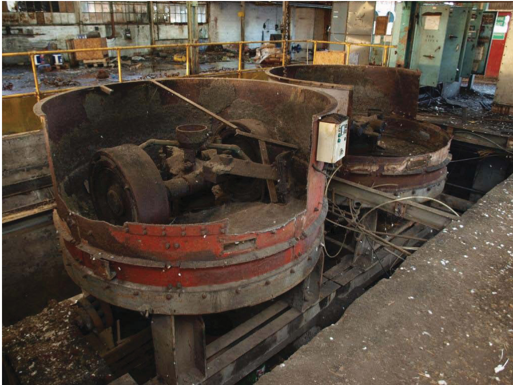
Plate 25. Detail view sand treatment machinery found at the north end of the eastern half of the Old Bronze Foundry (5).
