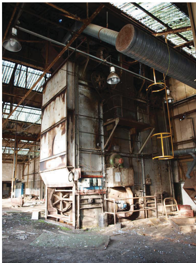
Plate 22. Oil fired oven in large space at south end of eastern half of Old Bronze Foundry (5).
