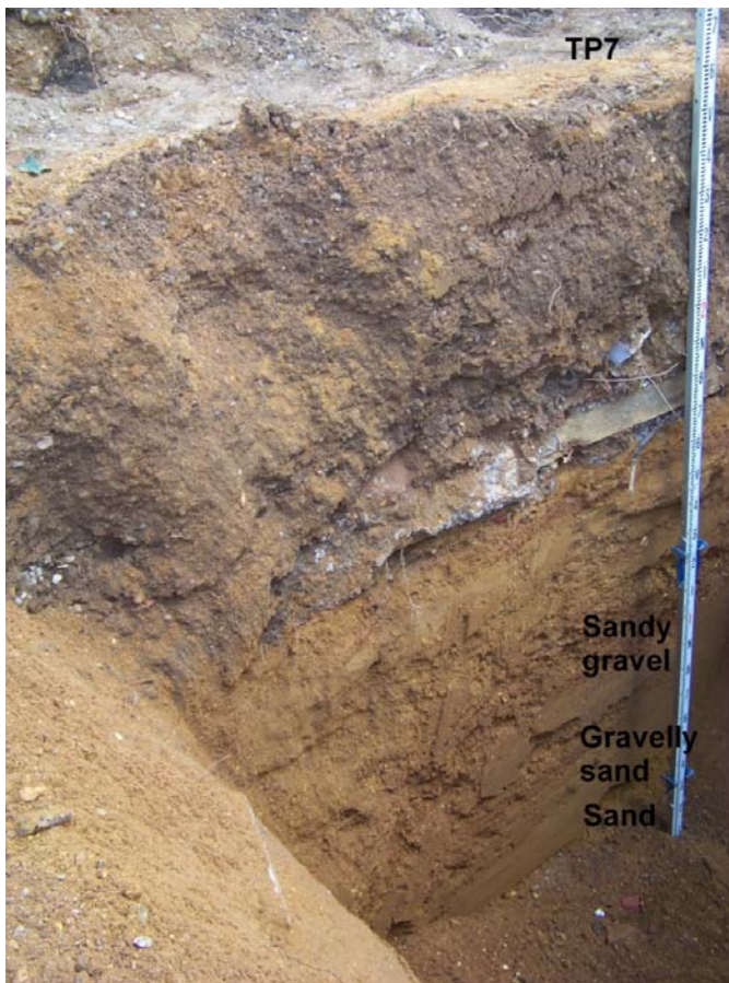
Figure G11: Trial Pit 7, Full Section, Oblique, North Face (south facing)
