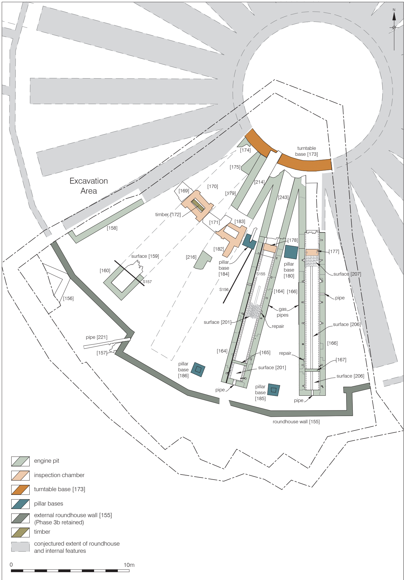
Figure 12 Phase 3c, Roundhouse modifications and additions 1:200 at A4
