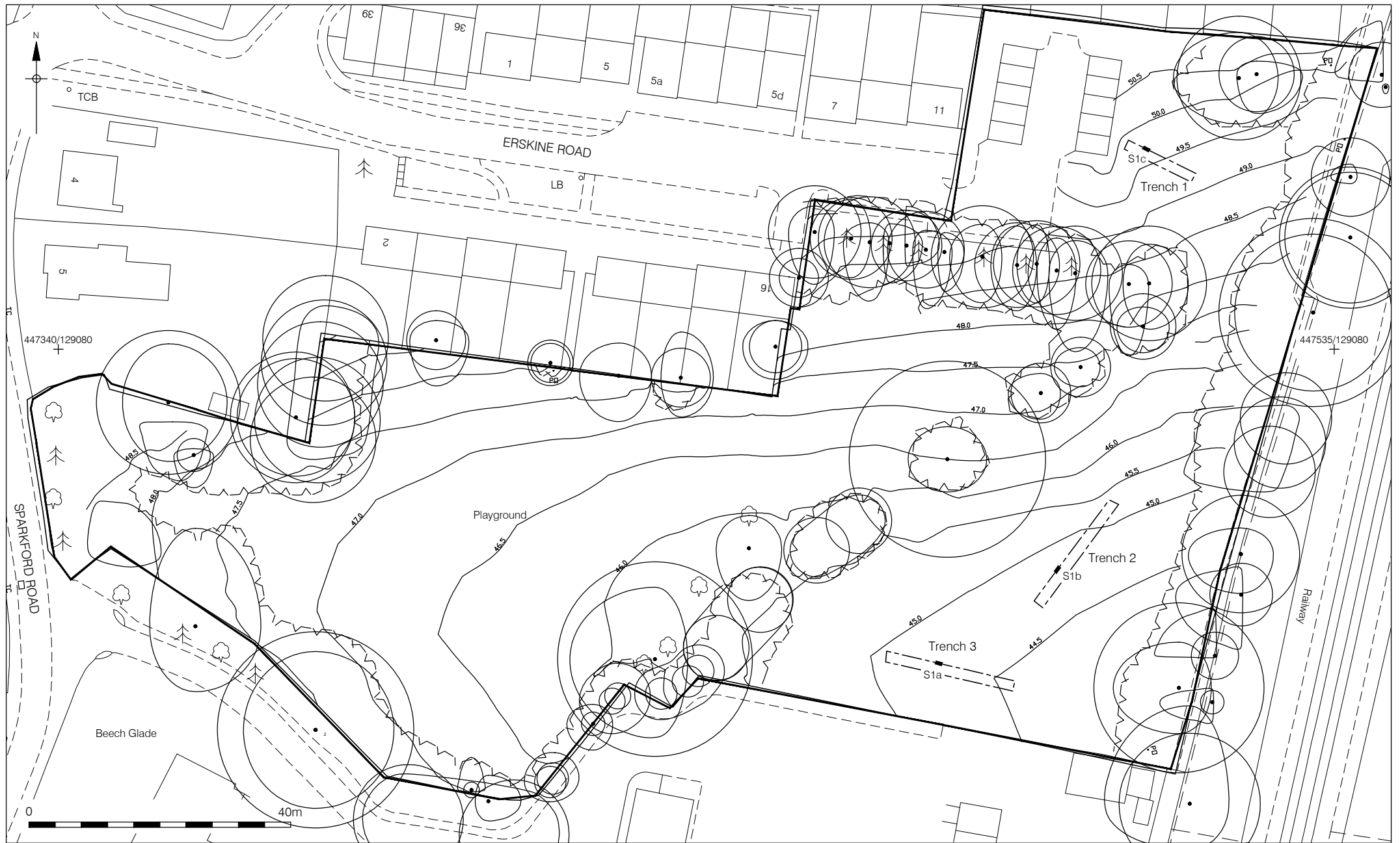
Figure 2 Trench Location rev 1 1:750 at A4
