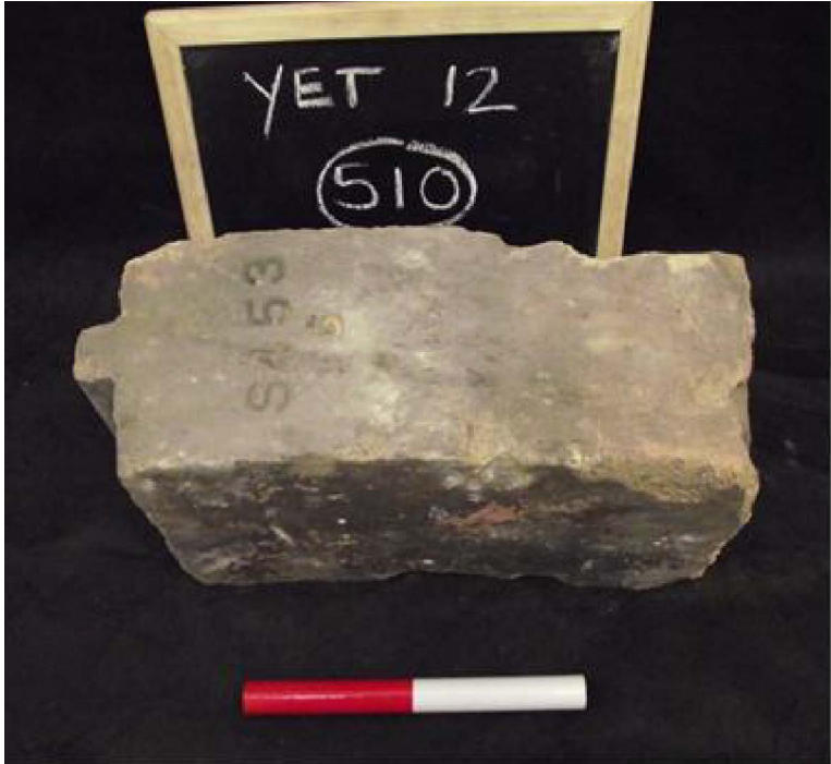
Plate 8-13 Curved firebrick with tongue from locomotive firebox, from RH2 (scale 0.20m)
