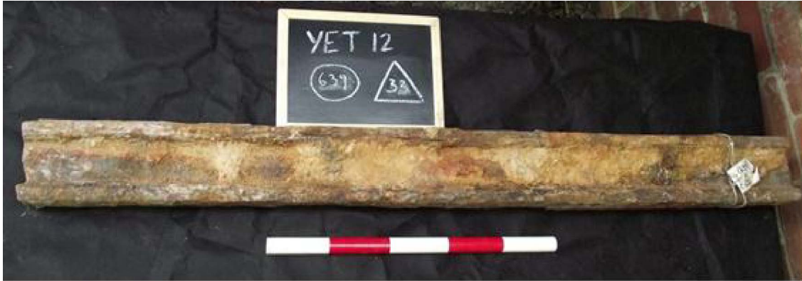
Plate 7-17 SF33 worn rail head from RH3 (scale 0.50m)
