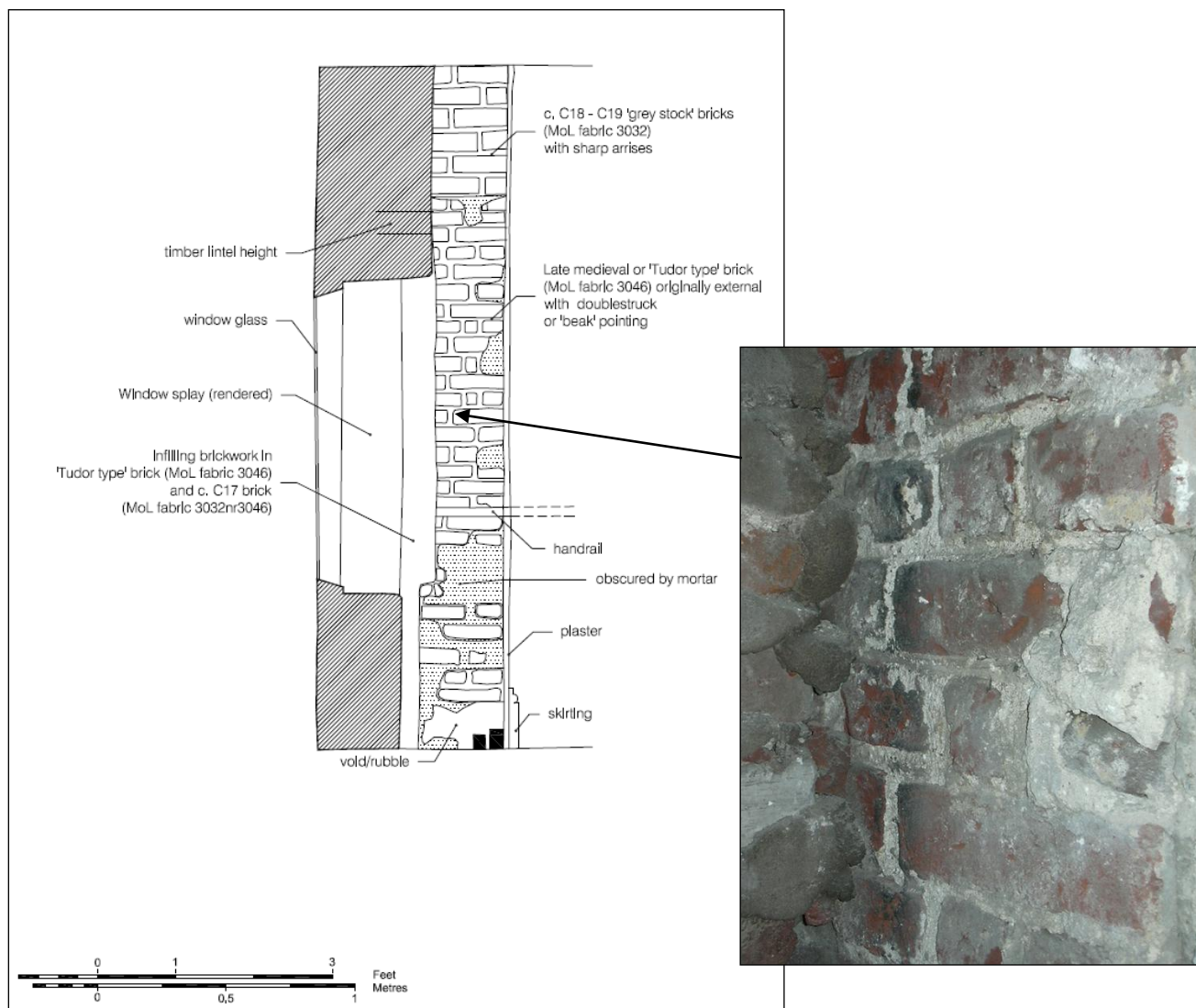
Figure 10: Late medieval or early Tudor brickwork with double-struck, or 'beak', pointing (Room 129)
