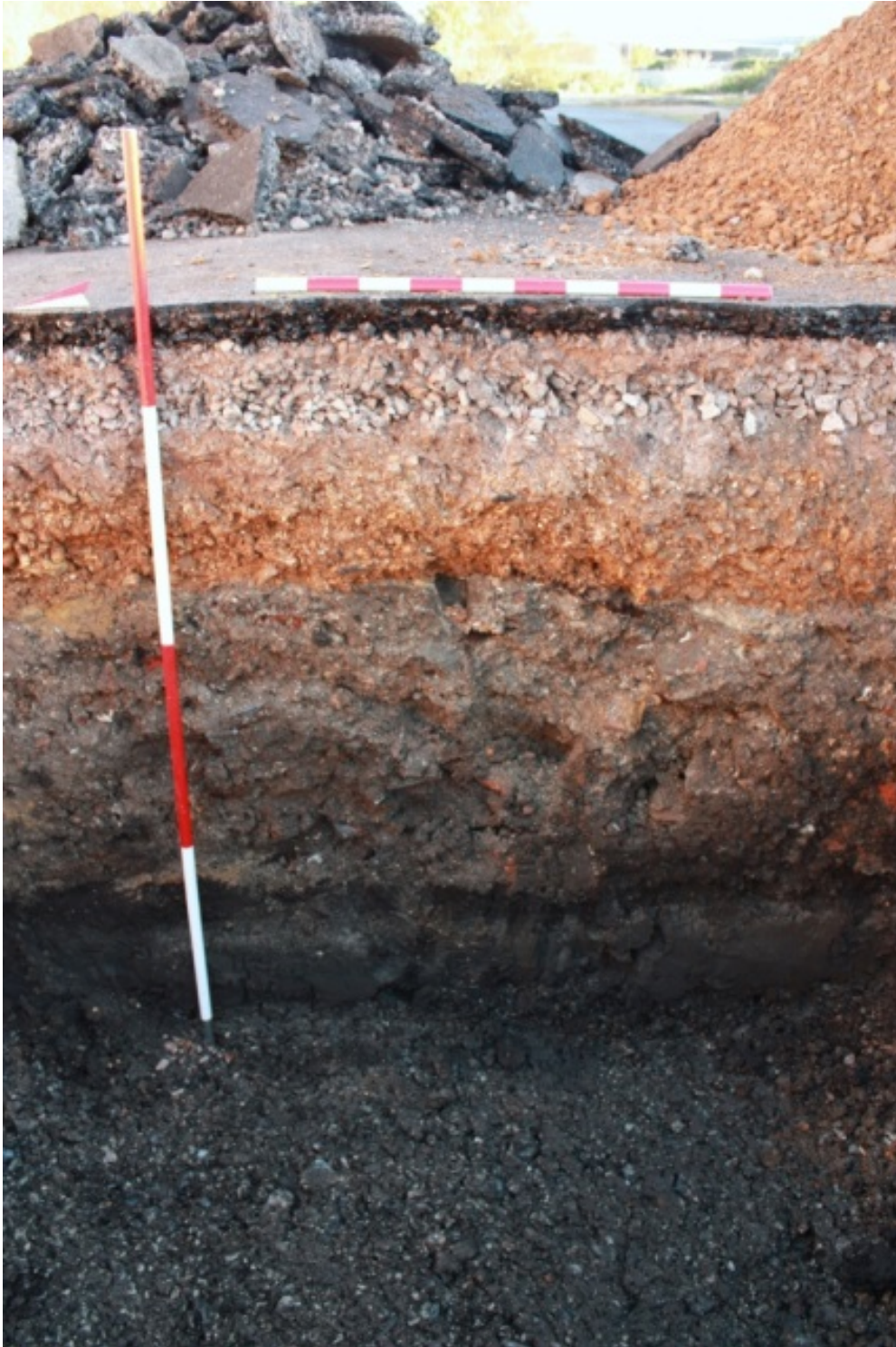
Plate 5. D2.2. Taken 22/11/13. TP3 view showing peat deposit [16] a dark thin band directly below layers of modern made ground and overlaying [17] an alluvial clayey sand sealing natural gravel [18]. Scales are 1m and 2m looking E.
