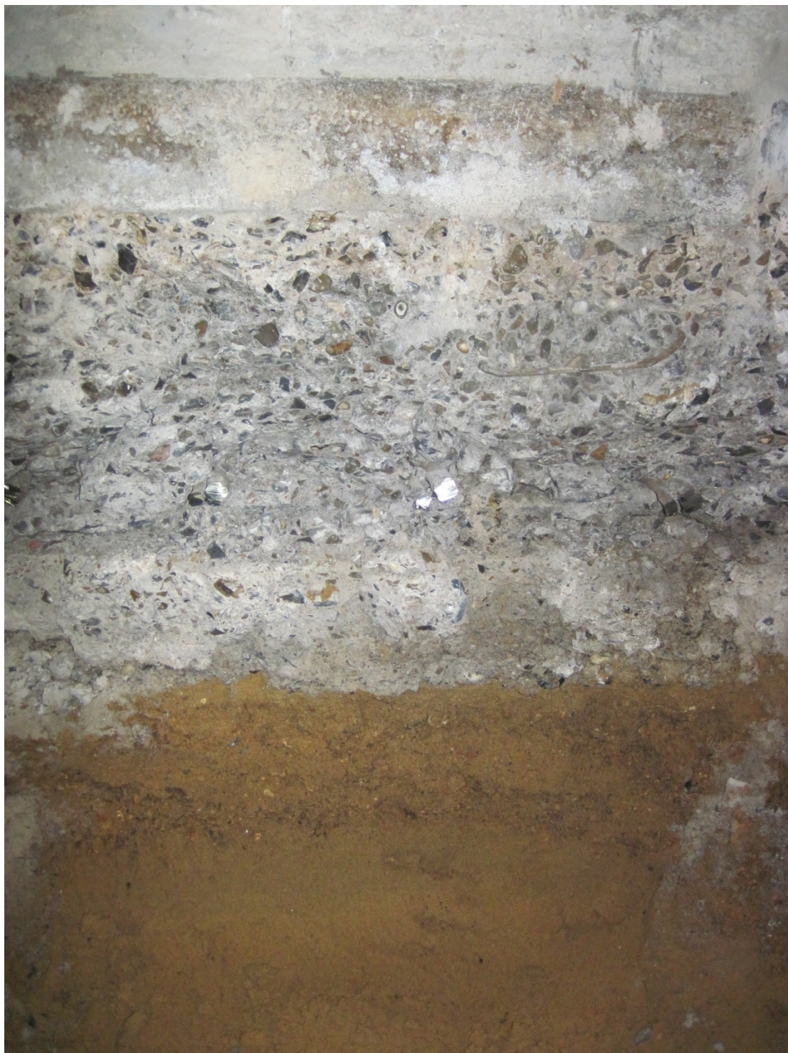
Plate 5 South West facing section in Test Pit 5; natural deposits immediately below concrete
