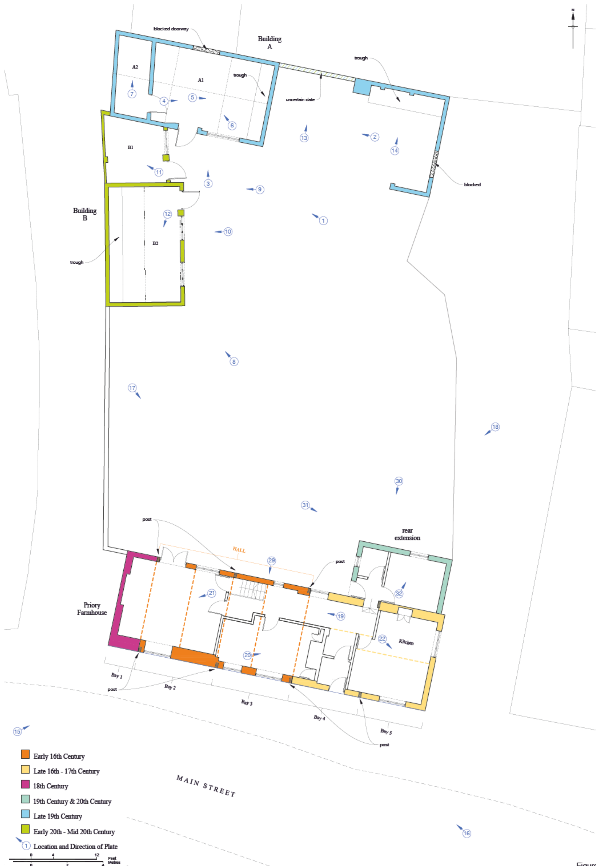
Figure 10 Ground Floor Plan of Buildings A & B and the Priory Farmhouse 1:125 at A3
