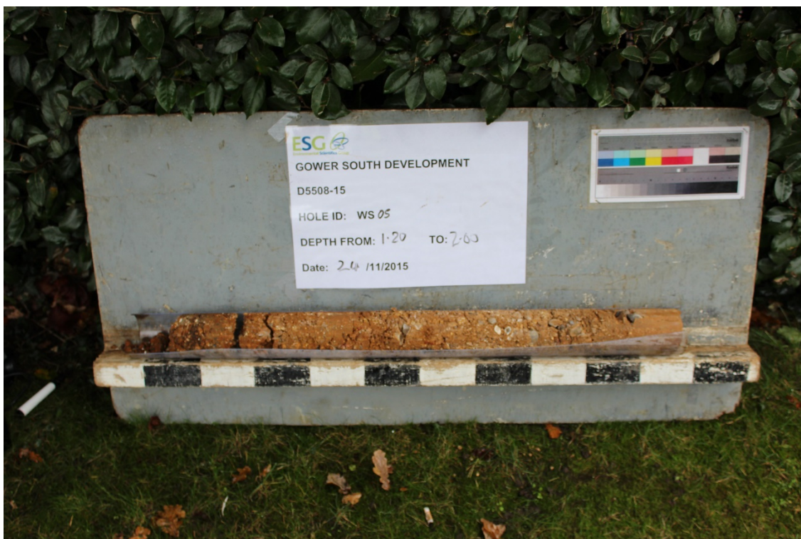
Plate 1 Core from WS05 showing interface between the made up ground and Brickearth
