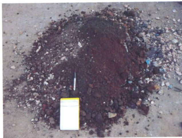
ARISINGS FROM INSPECTION PIT
