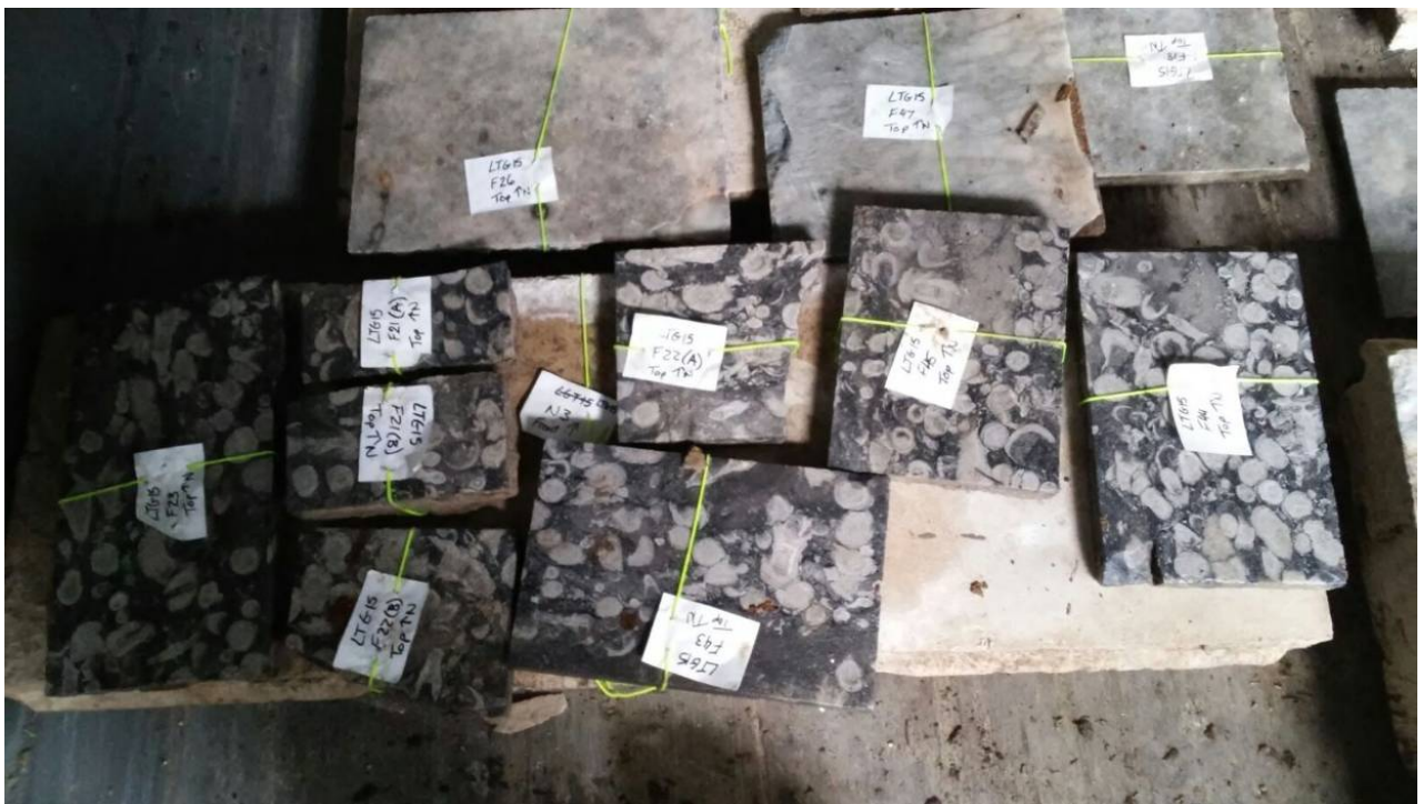
Plate 37 Ex-situ Frosterley and Carrara Marble tiles from the floor of the bath
