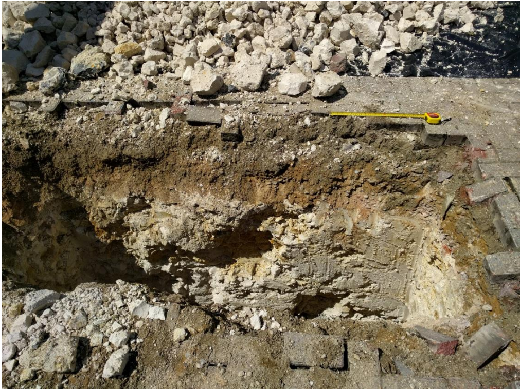
Plate 2 Southeast facing view of Test Pit 2; showing the top of chalk [3] overlain by concrete [8] and sealed by tarmac [1].
