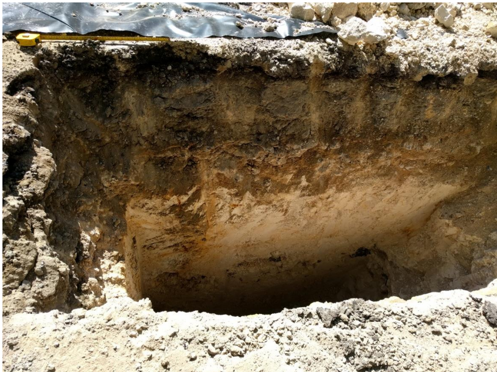
Plate 2 Southeast facing view of Test Pit 2; showing the top of chalk [3] overlain by concrete [8] and sealed by tarmac [1].
