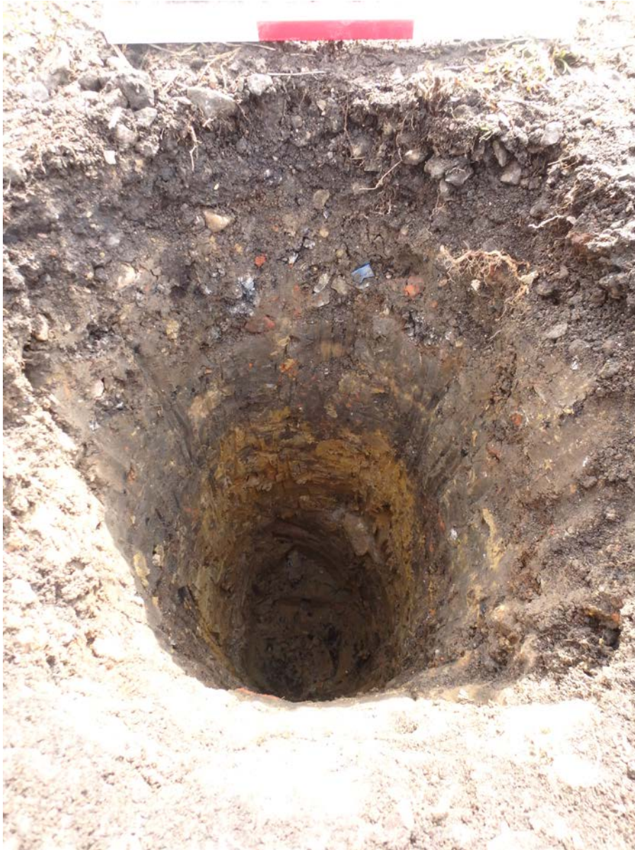
Plate 5 - NPIBH16 – Starter Pit, mixed made ground with clay below
