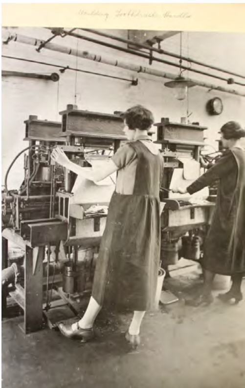
Plate 19: Moulding Toothbrush Handles (SRO Ref. HC 410/J1/2)
