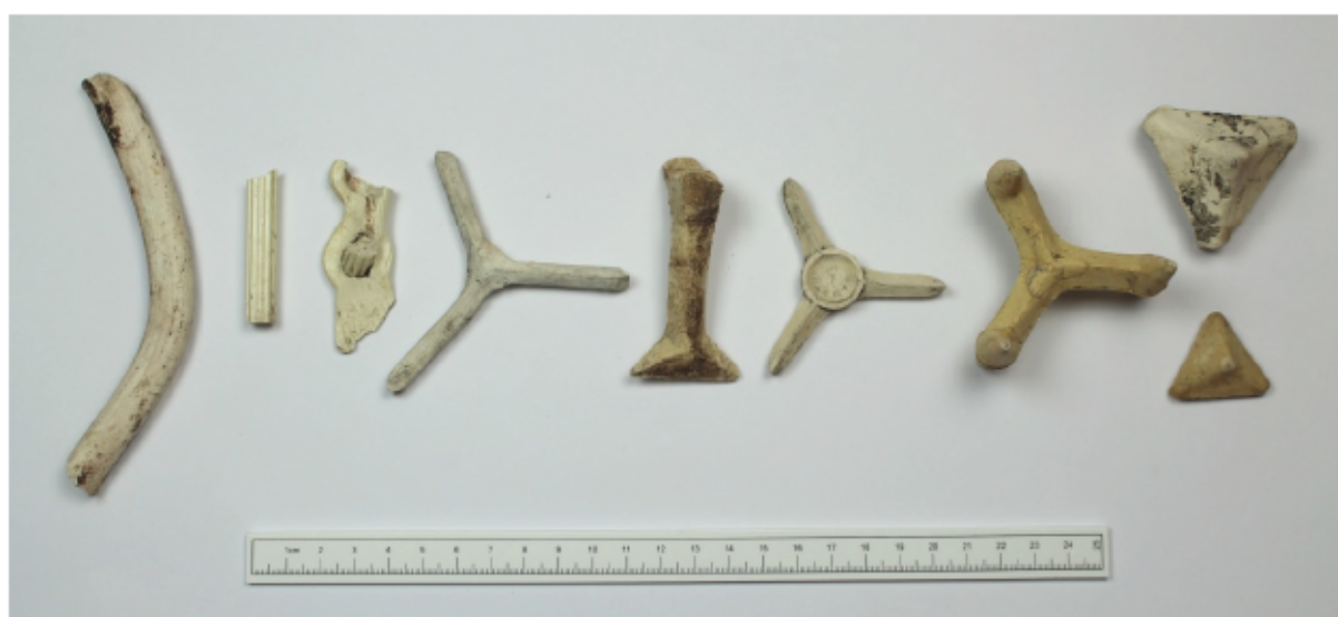
Figure 1: From left to right; one example of a handmade earthenware coil, one ridged separator used to separate plates within the kiln during glost firings, one separator wall attachment for within saggars walls (with separator still in situ), one biscuit state stilt with wedged feet for plate separation within saggars, one stilt with a 'fishtail' foot to separate deeper vessels such as
