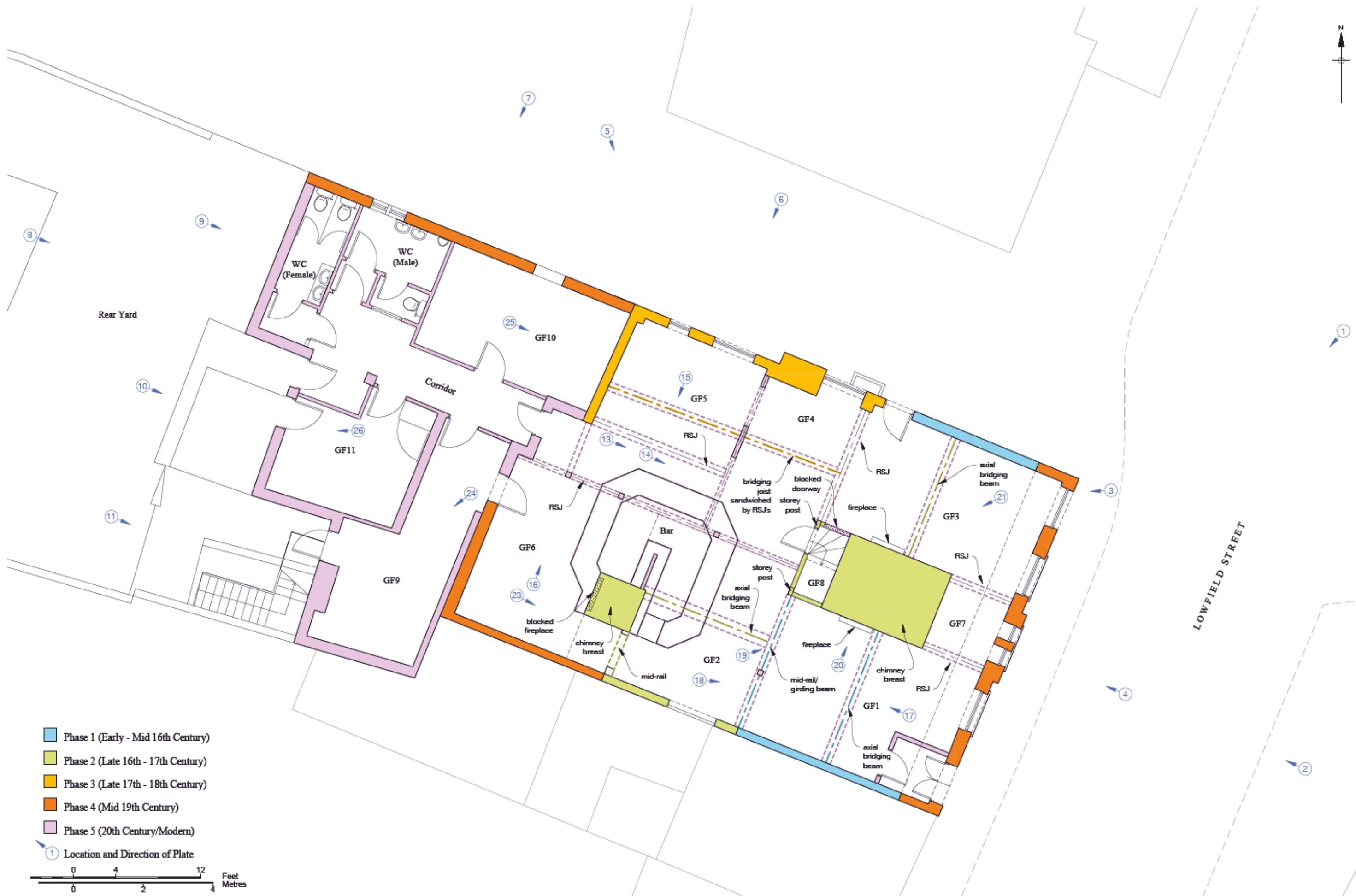
Figure 13 Existing Ground Floor Plan showing Phasing & Plate Directions 1:100 at A3
