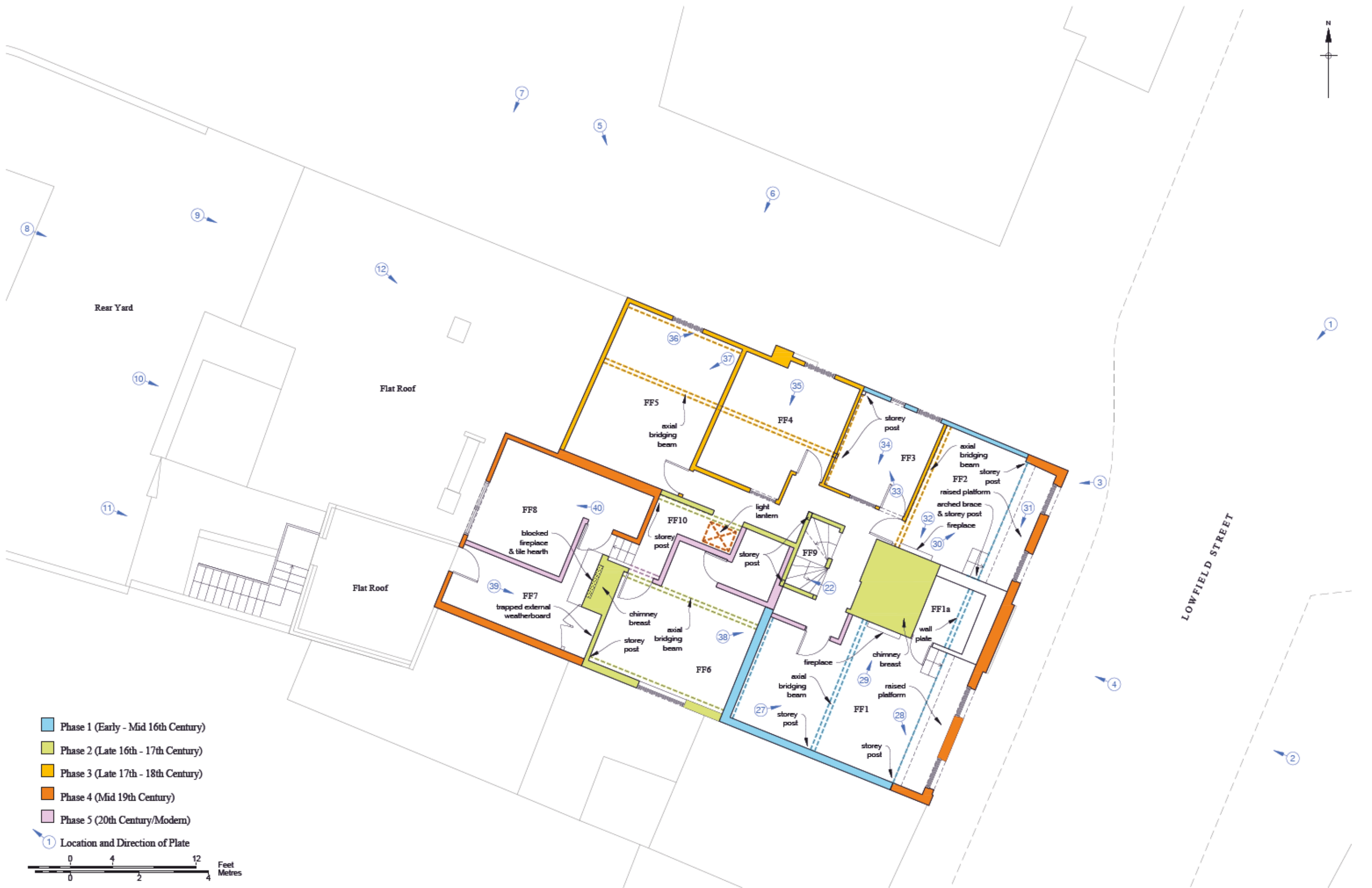
Figure 14 Existing First Floor Plan showing Phasing & Plate Directions 1:100 at A3
