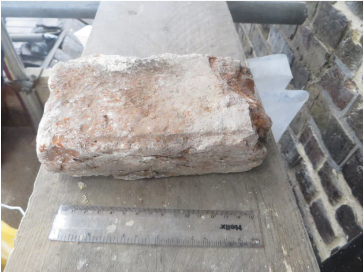
Plate 7: Tudor/Stuart brick from the north side of the east gable wall of the Queen's House
