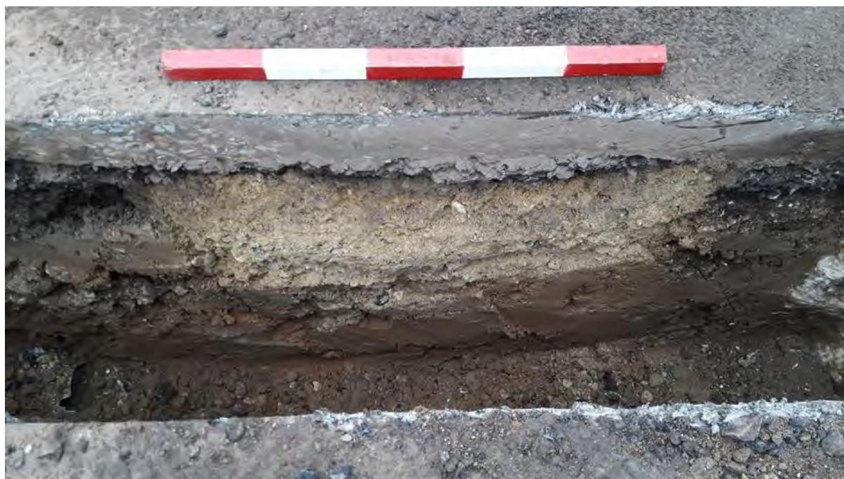
Plate 8 Sample section, 0.75m depth. Pale gravel fills of recent service cut, looking east
