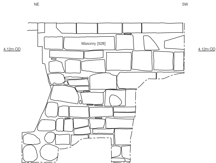
Section 18 Main excavation/Flying buttress of the Chapter House North west Facing
