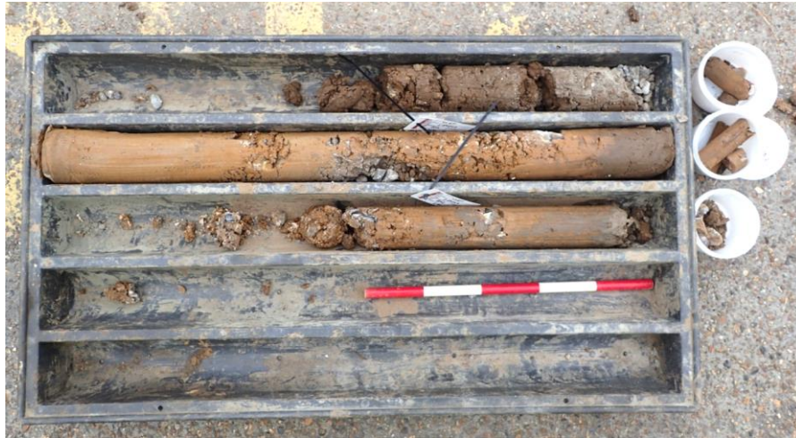
Plate 6: Borehole 2 core showing 'plough soil layer [4] at top with brick-earth [5] in the slot below terminating in a compacted flint nodule layer (just above the scale) [6].
