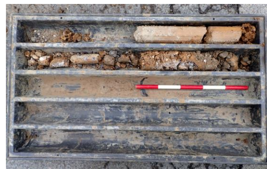
Plate 7a: Location of Borehole 3 immediately west of the Canning Flex Warehouse, view to Plate 7b: BH3 core showing brick-earth [1] at top with increasing compacted flint [3]
