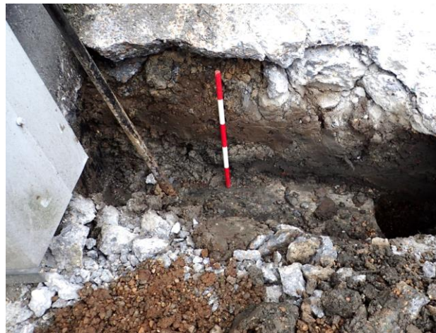
Plate 4b: View to SE of Test Pit 6. Only a small aperture was made next to the concrete stepped foundation restricting the observation of the lower layers. Only made ground layer [18] is visible. Scale 0.5m
