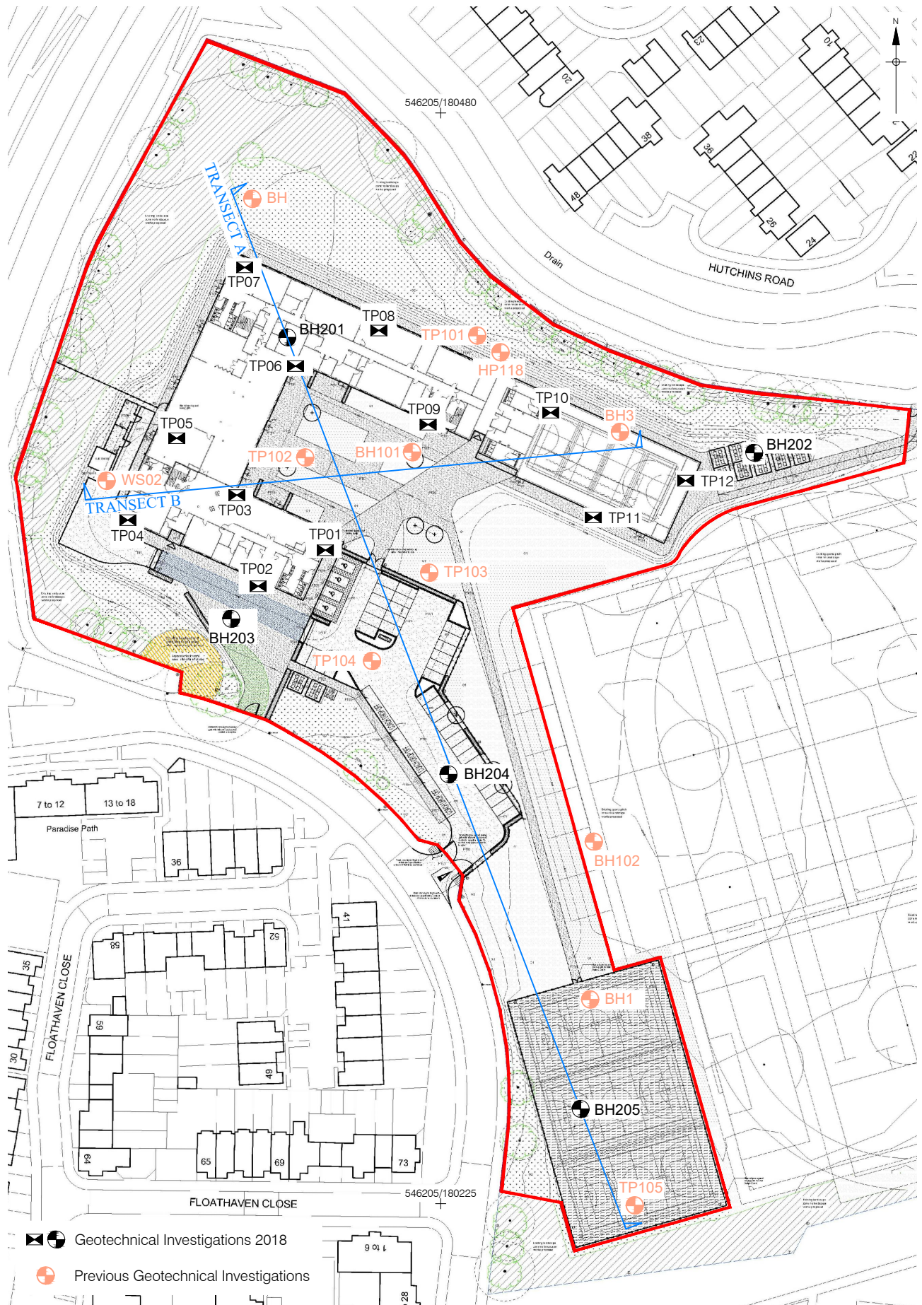
Figure 5 Borehole and Test Pit Locations overlain on Masterplan 1:1,250 at A4
