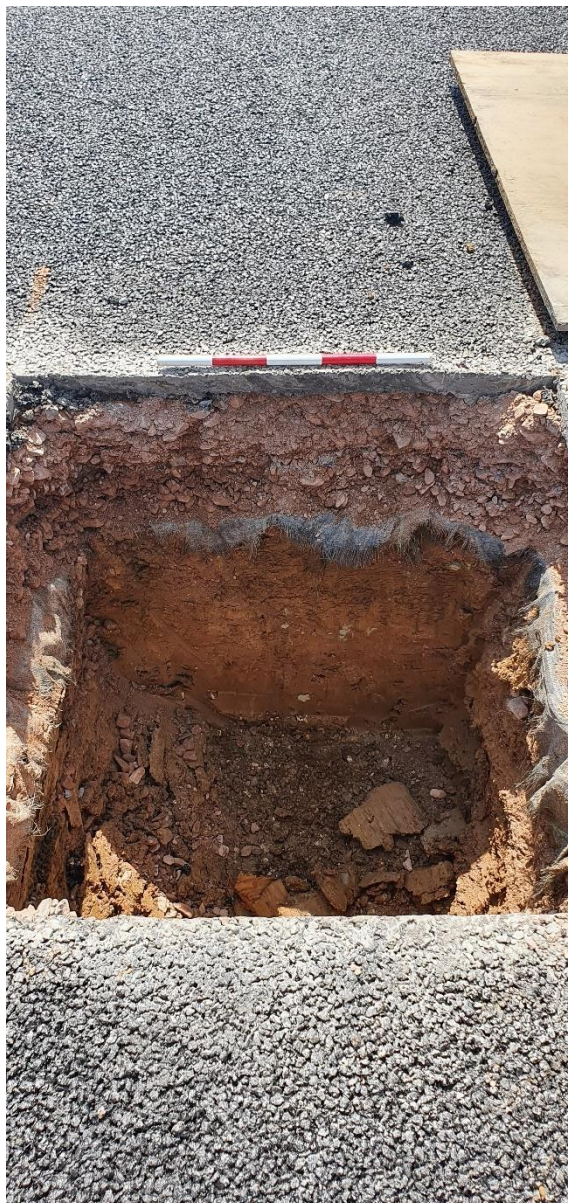
Plate 9: North facing Section 10 within the north-eastern goal post, natural gravels [37] can be seen at the very bottom of the slot c1.10m bgl; Scale 0.50m
