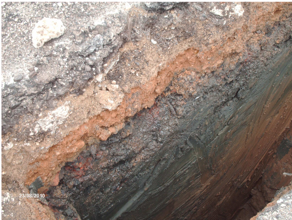
Figure 1Plate 10; Test pit 1013, looking SW, shows natural depositional sequence, including alluvium and topsoil, overlain beneath post-medieval levelling deposits.
