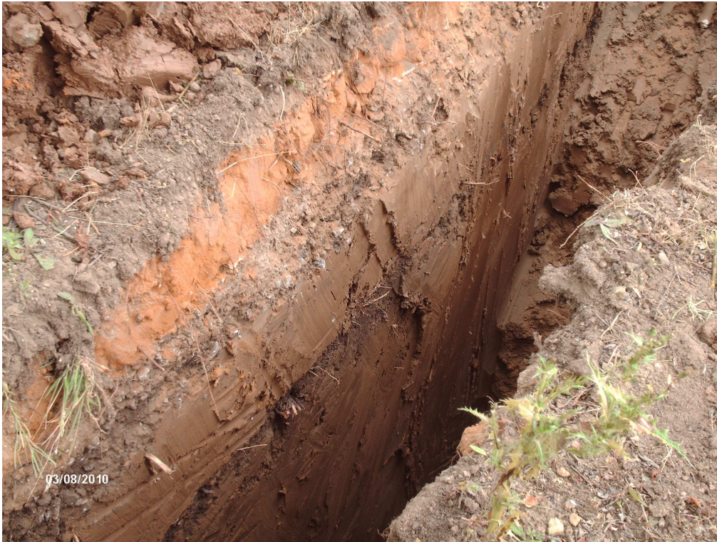
Plate 3; Test pit 2013, looking NE, shows natural sequence, including buried topsoil, overlain by post-medieval levelling deposits.
