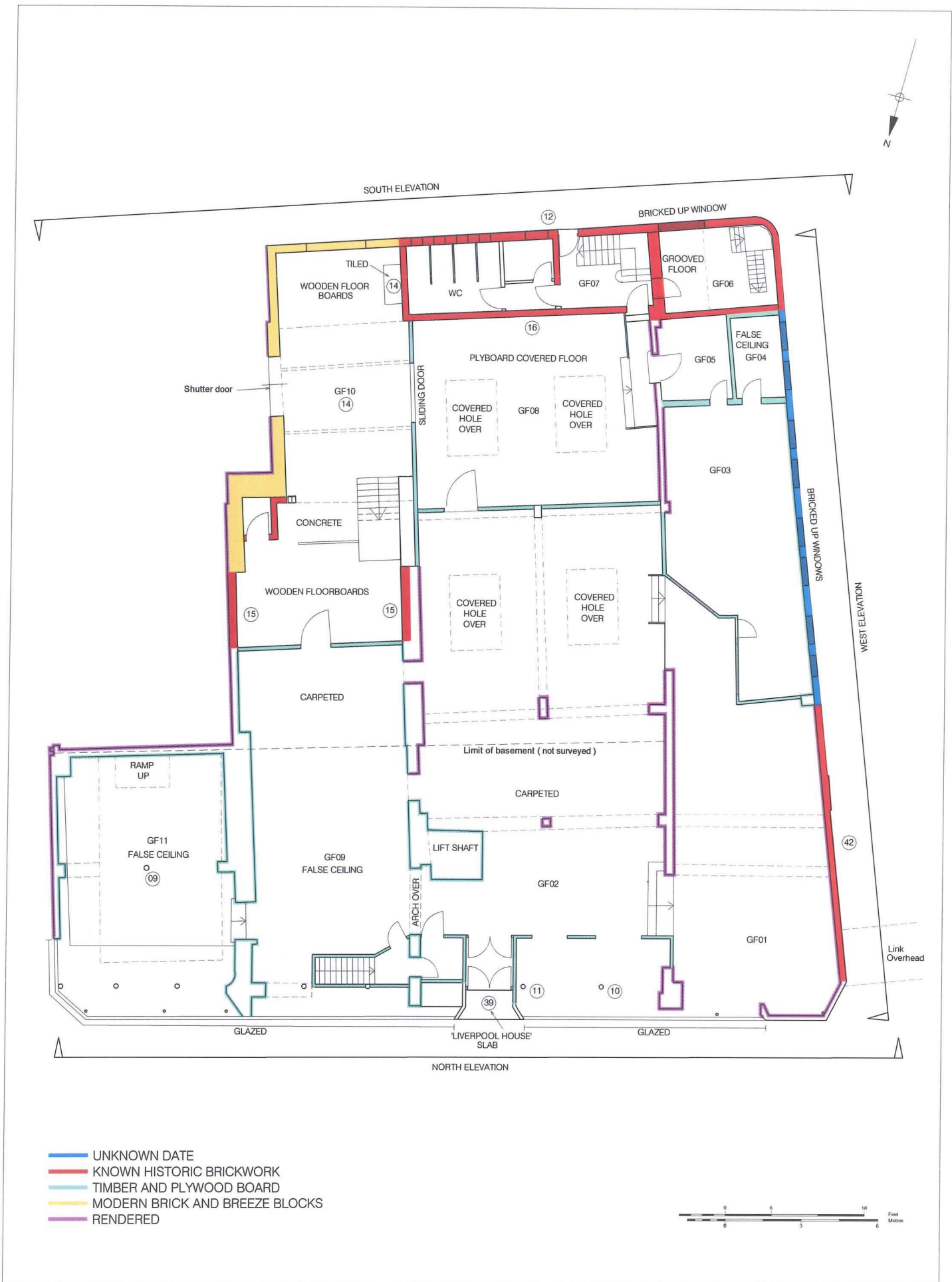
Figure 14 Ground Floor Plan showing areas of construction and important features (ref. Appendix 1) 1:200
