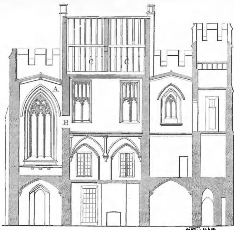
FIG. 24. BROUGHTON CASTLE, VERTICAL SECTION THROUGH THE FOURTEENTH-CENTURY EASTERN BLOCK.
