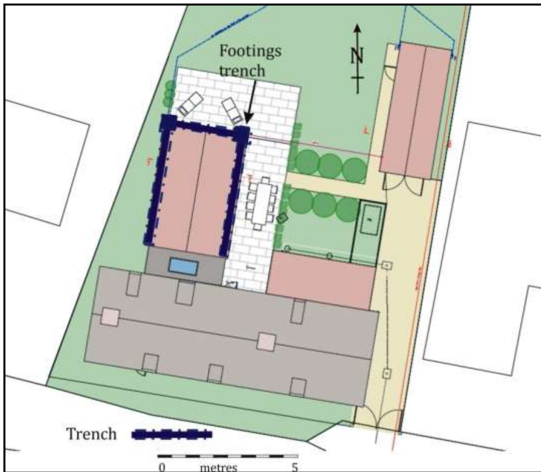
Figure 5. Overall plan of house with footings trench
