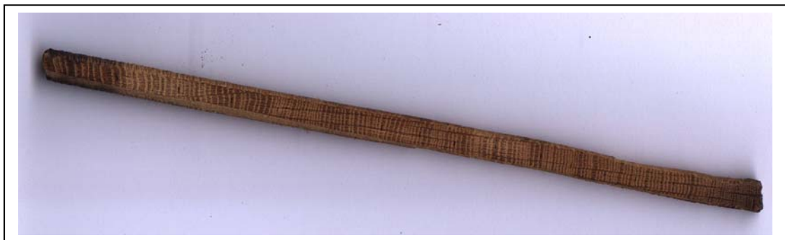
Core sample MUK-A01 from the south blade of the cruck truss. Although felled in 1439, the tree from which this sample is derived probably began growing as early as 1170.
