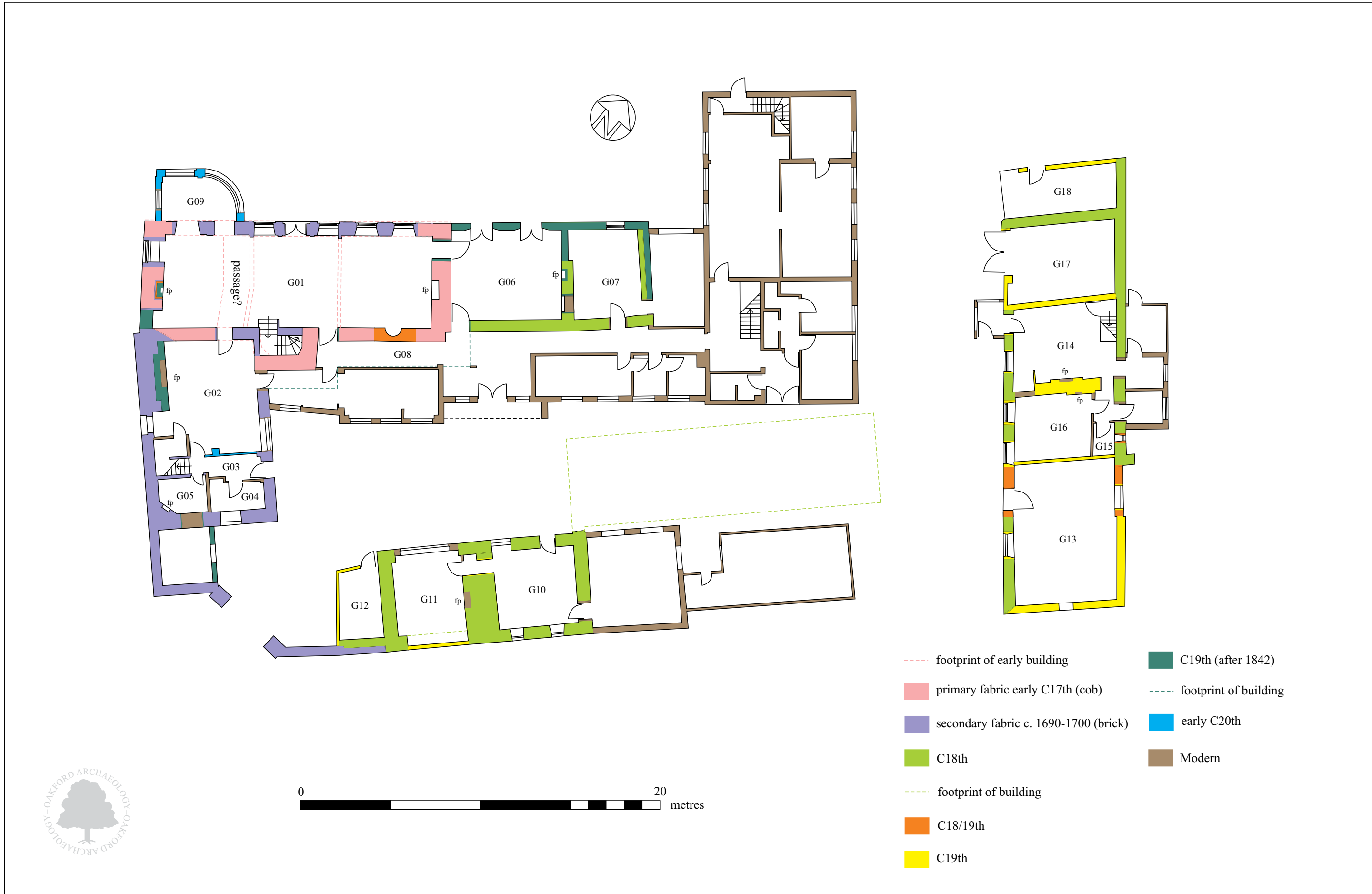
Fig. 9 Plan of ground floor showing location of observations during renovation work and suggested phases of development.
