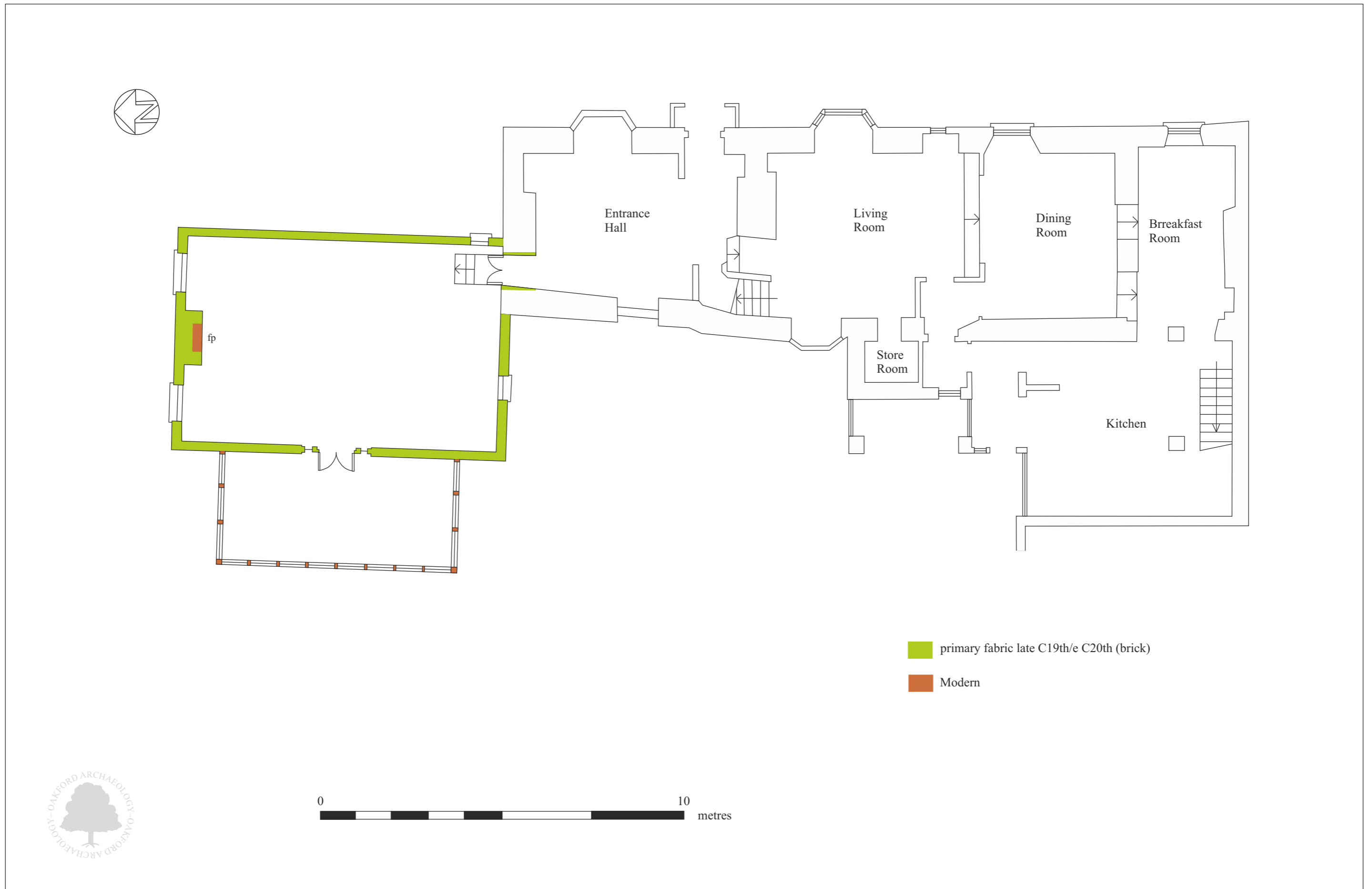
Fig. 8 Plan of ground-floor showing location of observations and suggested phases of development.
