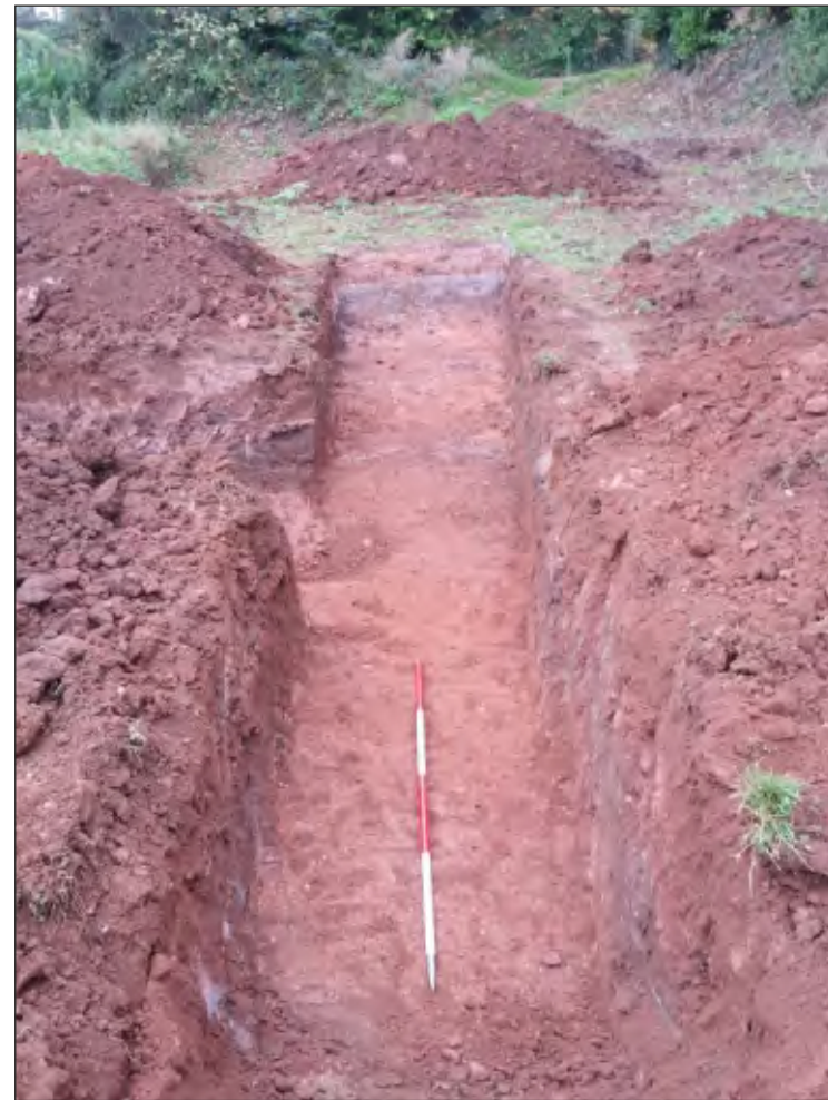
Pl. 4 General view of Trench 2 showing depth of modern made ground (200). 2m scale. Looking southwest.
