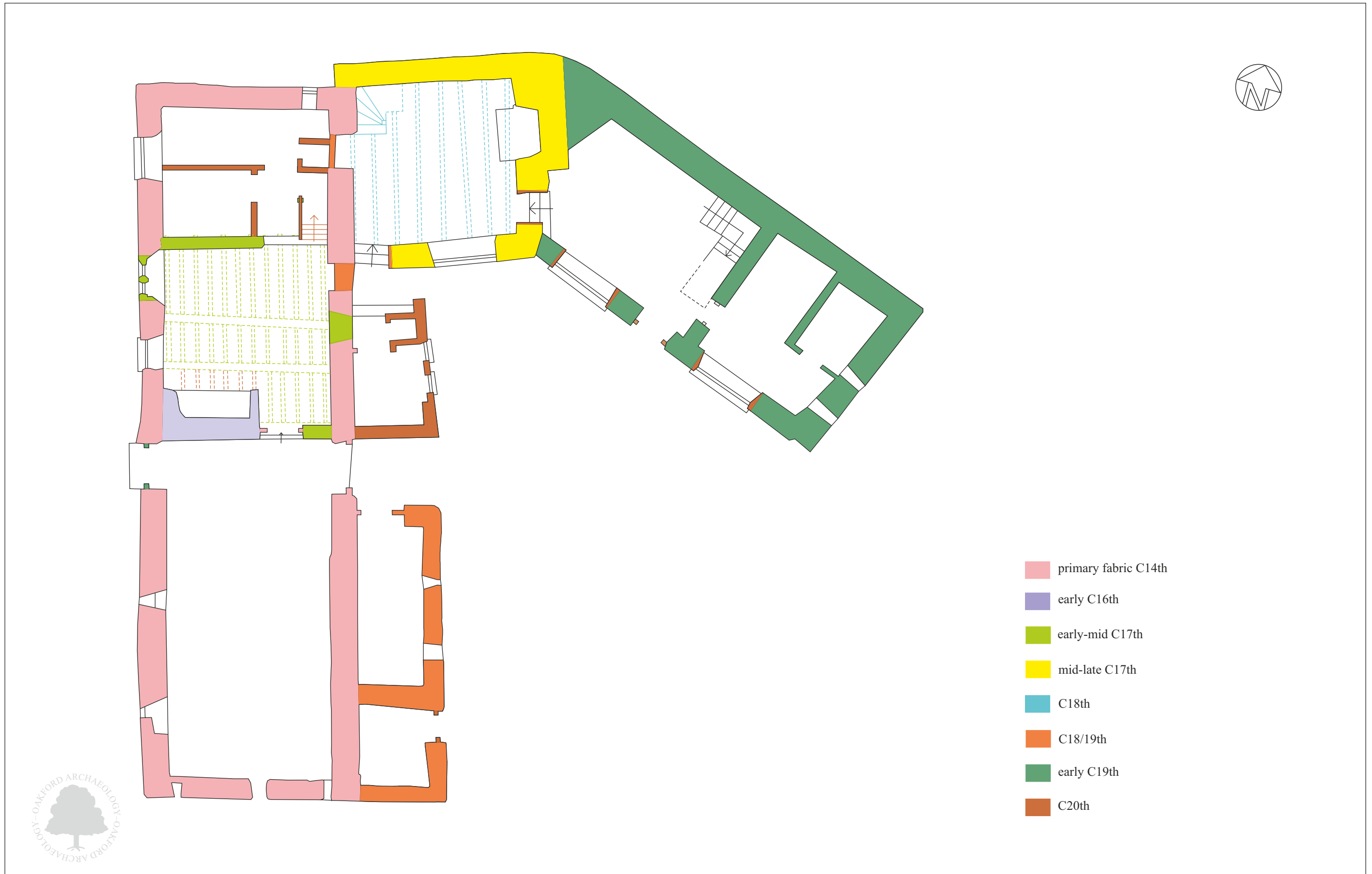
Fig. 4 Plan of ground floor showing location of observations during renovation work and suggested phases of development.
