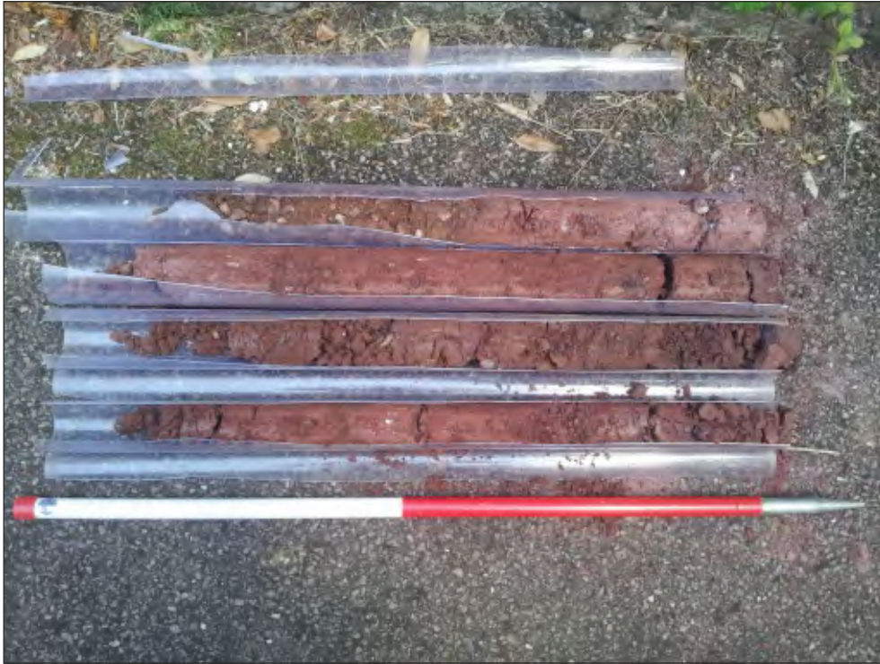
Pl. 11 Borehole 6 showing deposit sequence with buried soil (bottom left). 1m scale.
