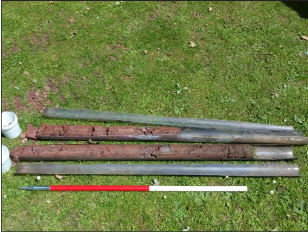
Pl. 7 Borehole 5a showing deposit sequence. 1m scale.
