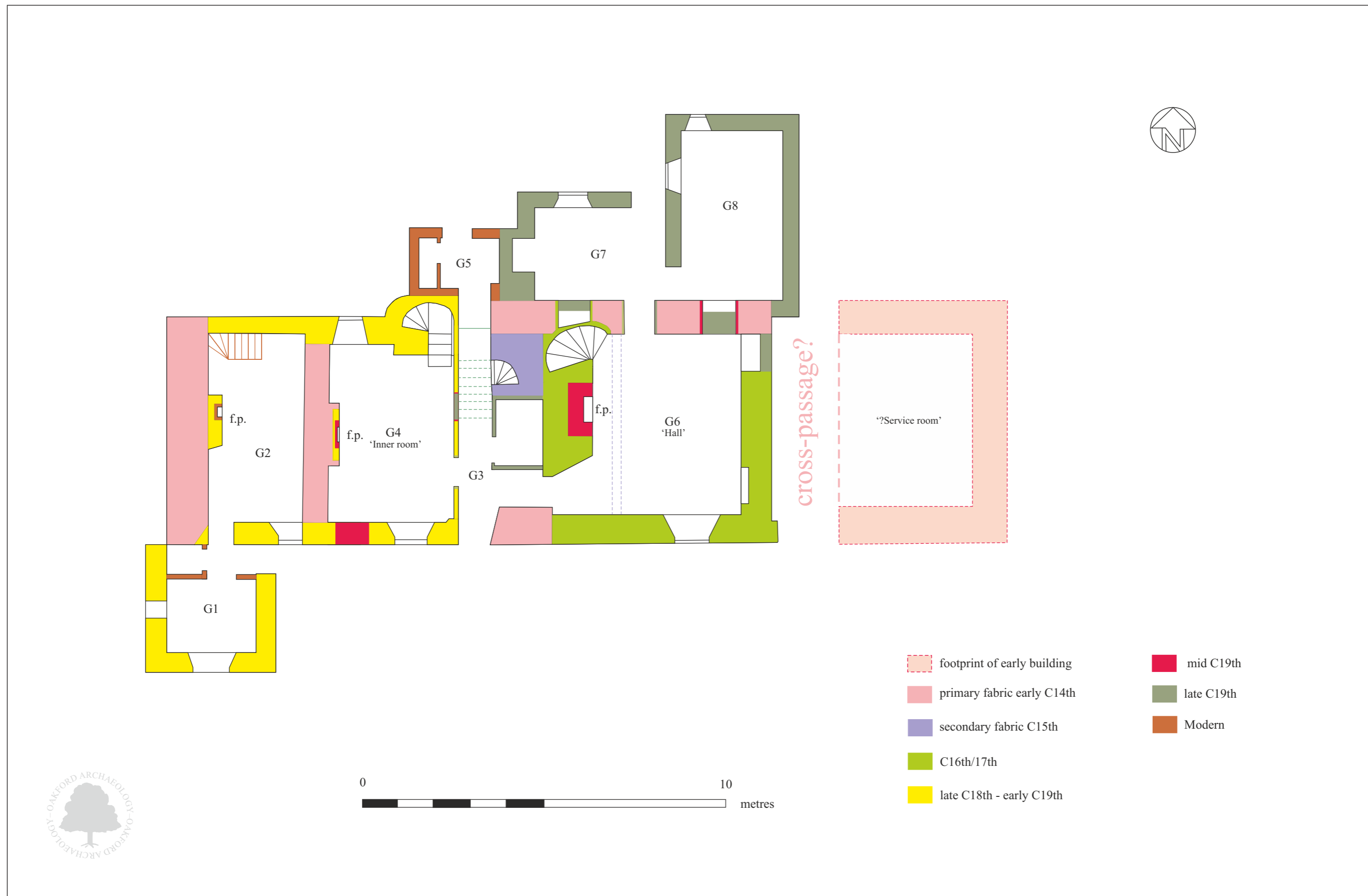
Fig. 5 Plan of ground floor showing location of observations during renovation work and suggested phases of development.
