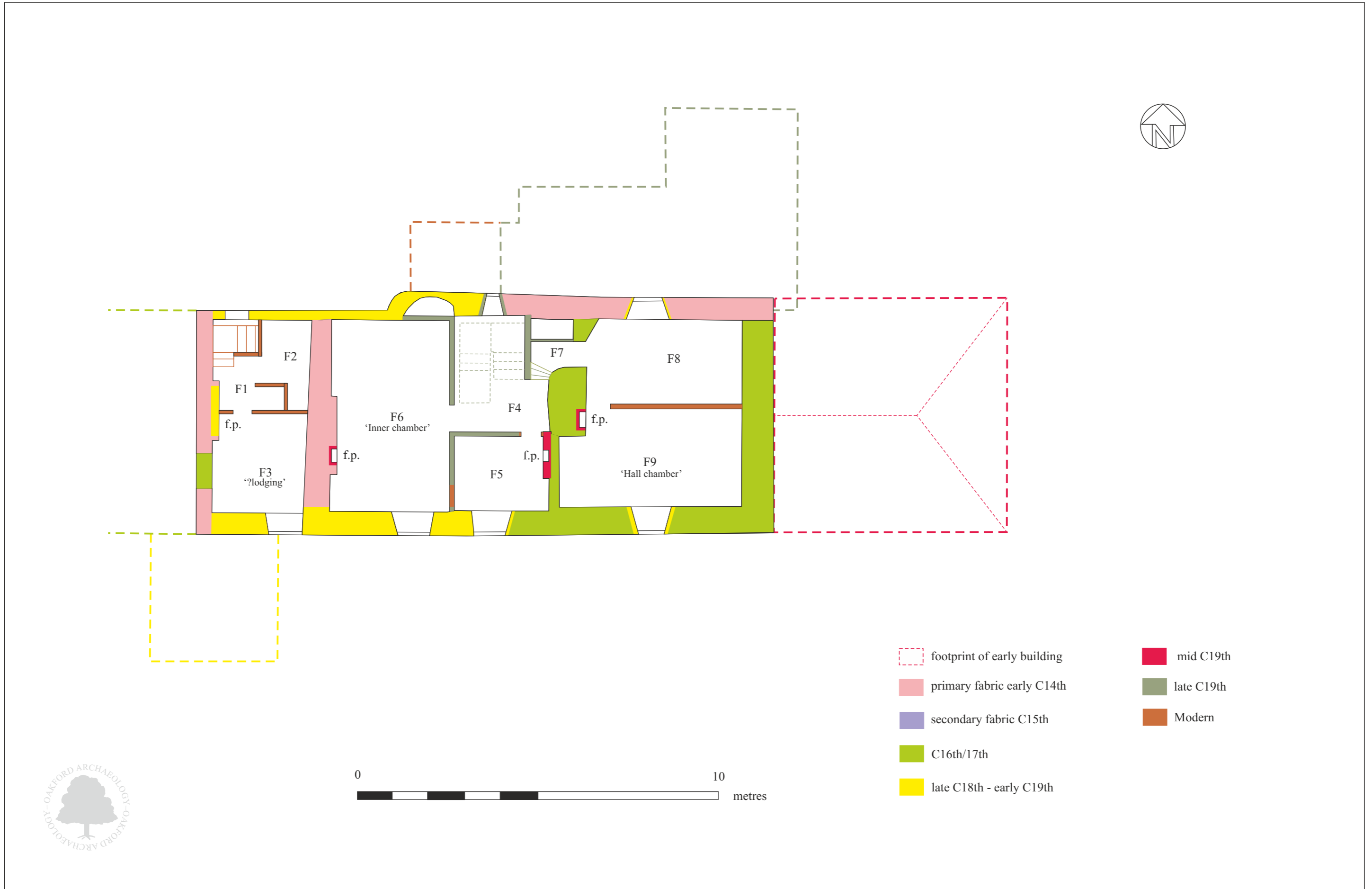
Fig. 7 Plan of first floor showing location of observations during renovation work and suggested phases of development.
