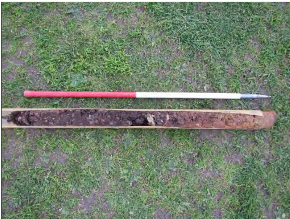
Pl. 2 Borehole 1 showing deposit sequence between 38.87-37.87m AOD (left to right). 1m scale.
