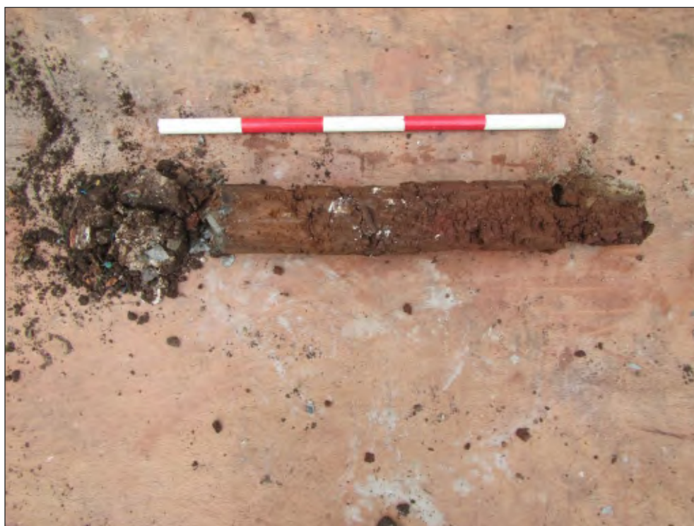
Pl. 8 Borehole 4 showing deposit sequence between 38.31-37.71m AOD (left to right). 1m scale.
