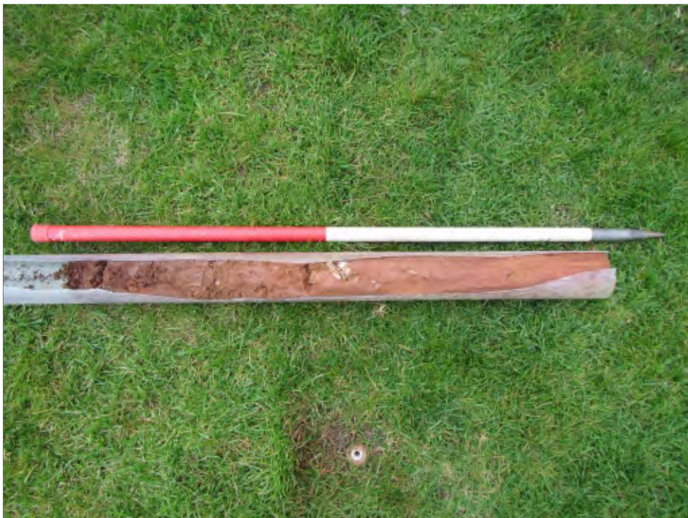
Pl. 4 Borehole 2 showing deposit sequence between 37.70-36.70mAOD (left to right). 1m scale.
