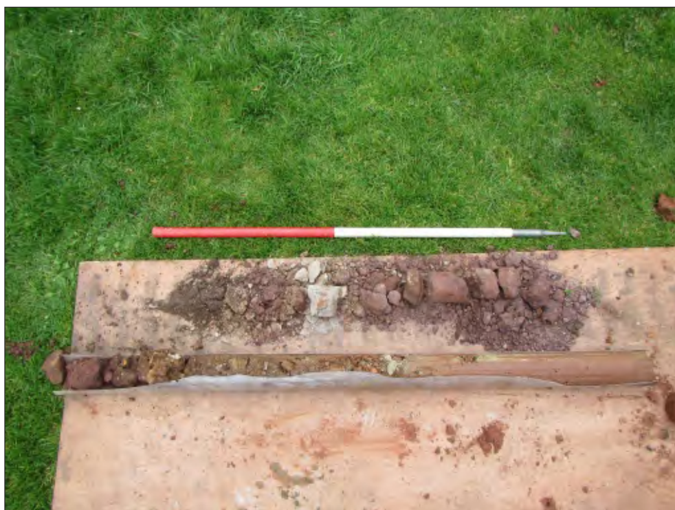
Pl. 6 Borehole 3 showing deposit sequence between 39.12- 38.62mAOD (top) and 38.62 - 37.62mAOD (bottom). 1m scale.
