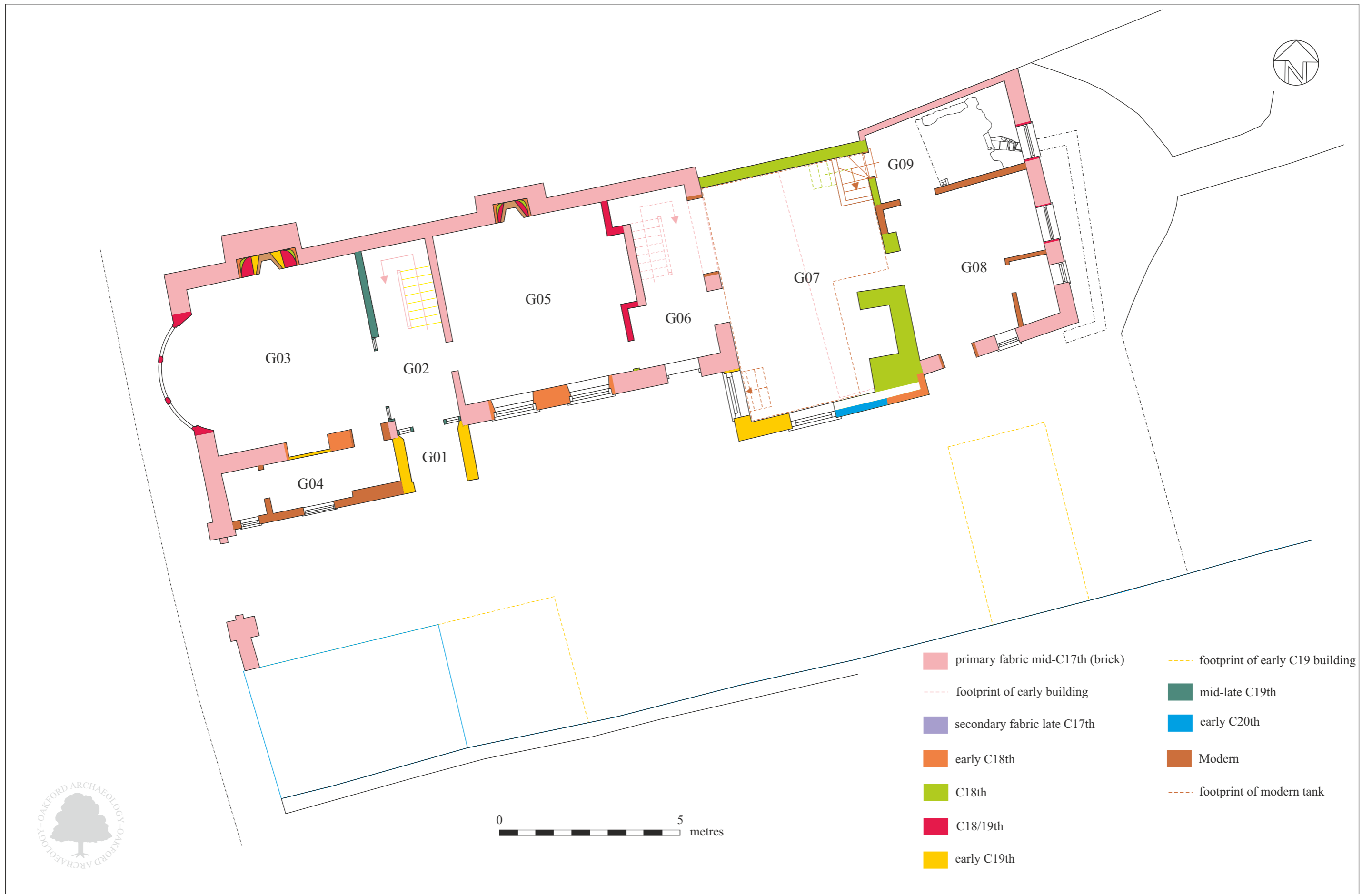
Fig. 16 Plan of ground floor showing location of observations during renovation work and suggested phases of development.
