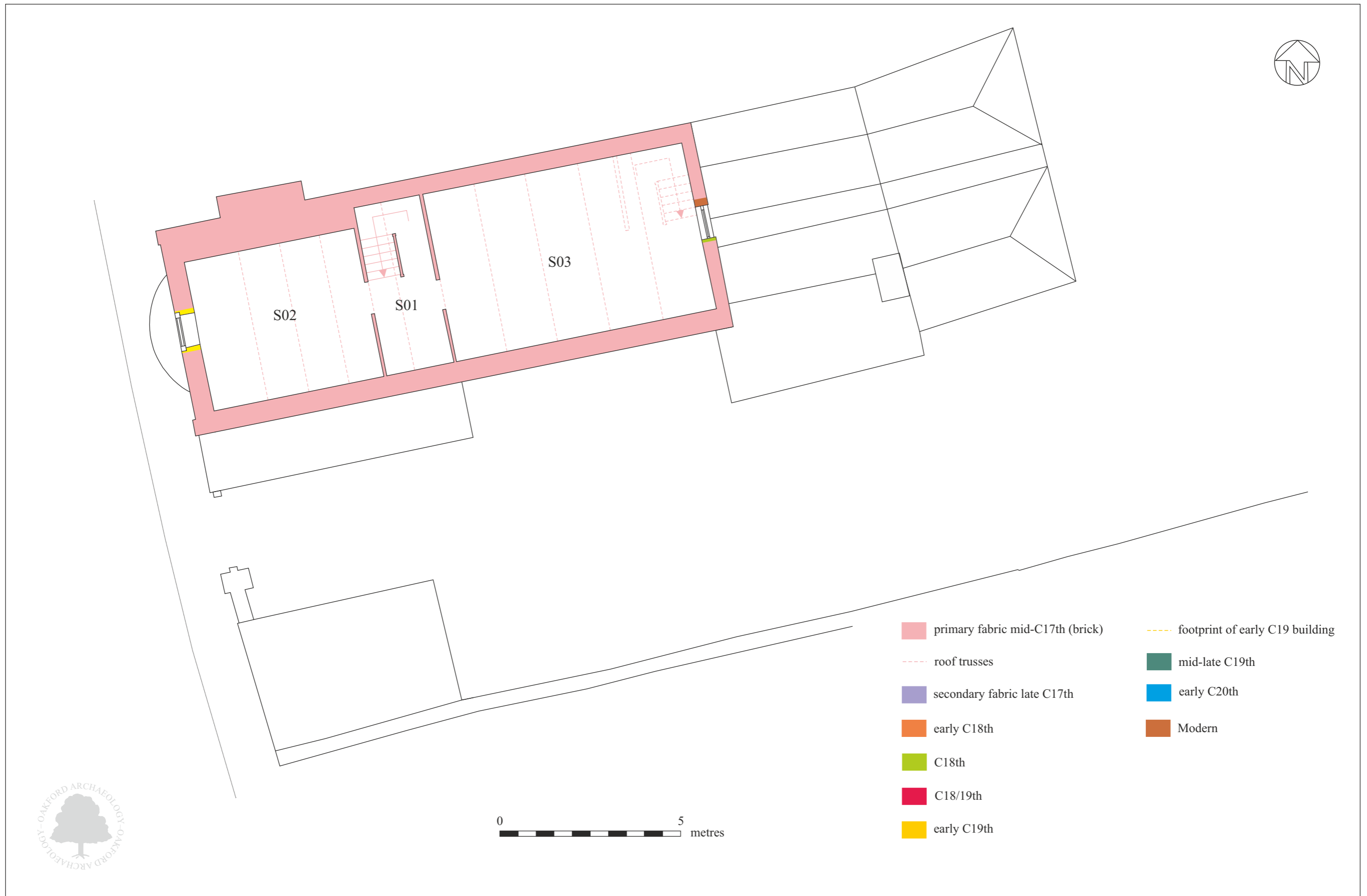
Fig. 20 Plan of the attic storey showing location of observations during renovation work and suggested phases of development.
