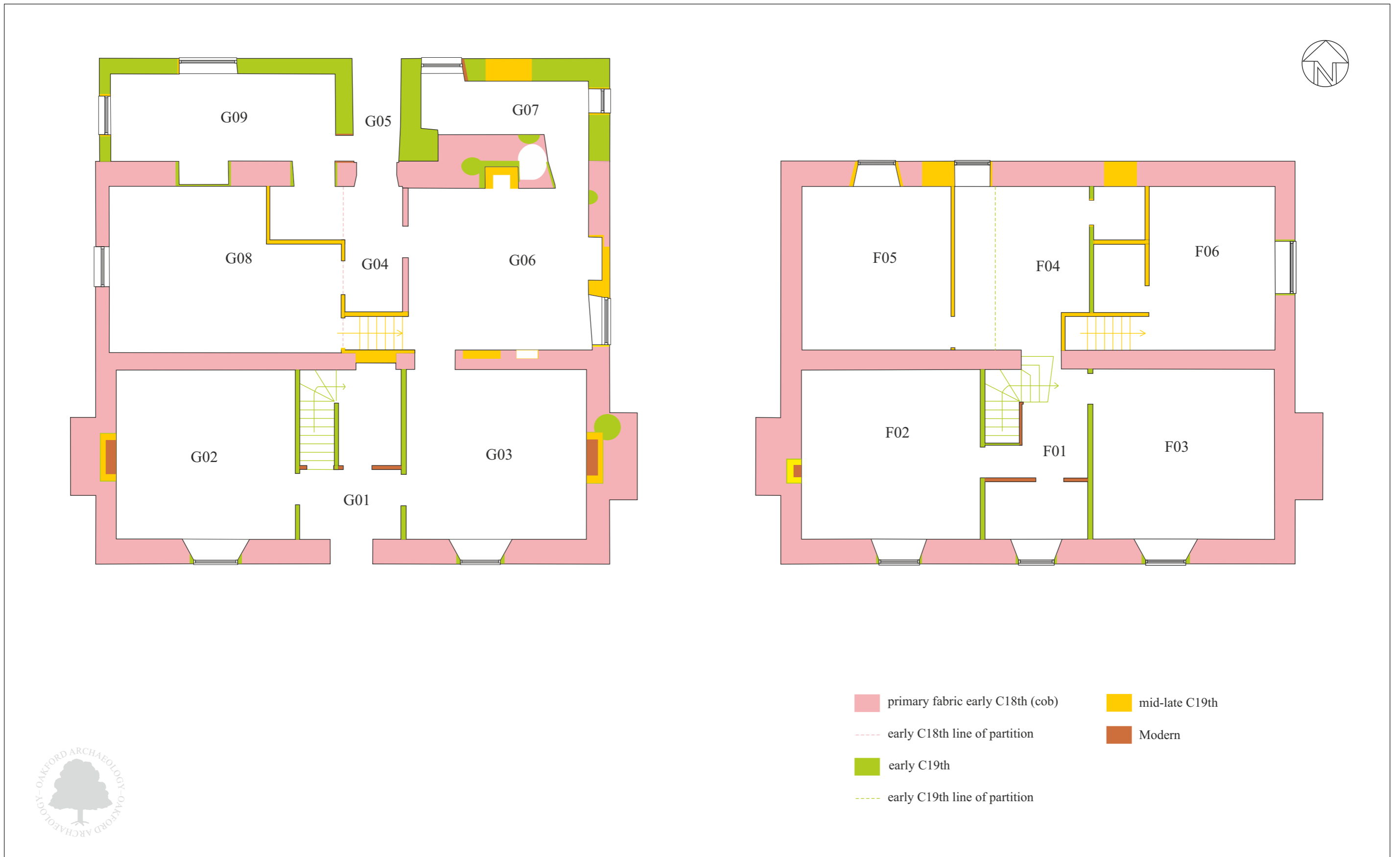
Fig. 7 Plan of ground- and first-floor showing location of observations and suggested phases of development.
