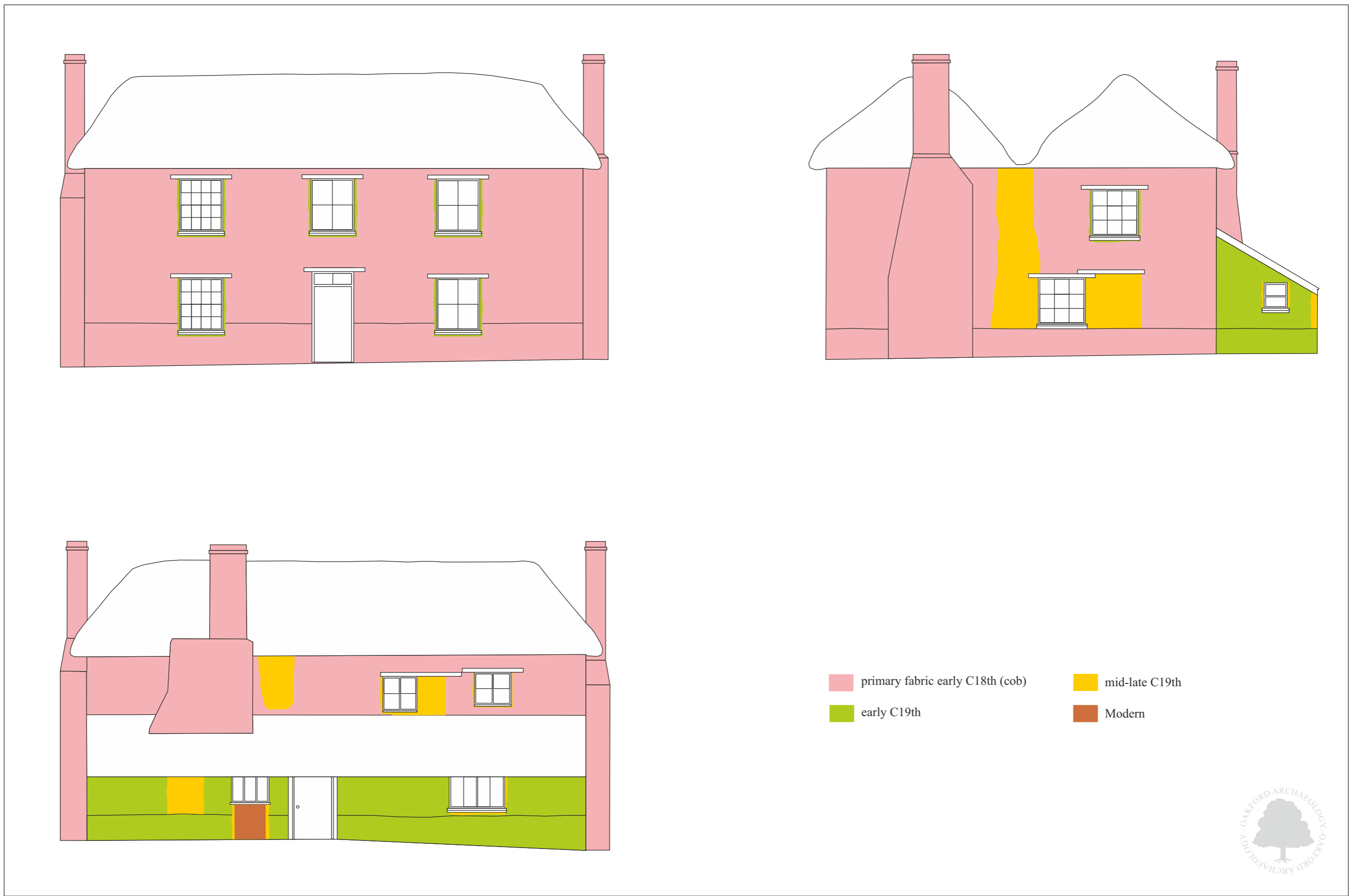
Fig. 6 External elevations (south, east and north) showing location of observations and suggested phases of development.
