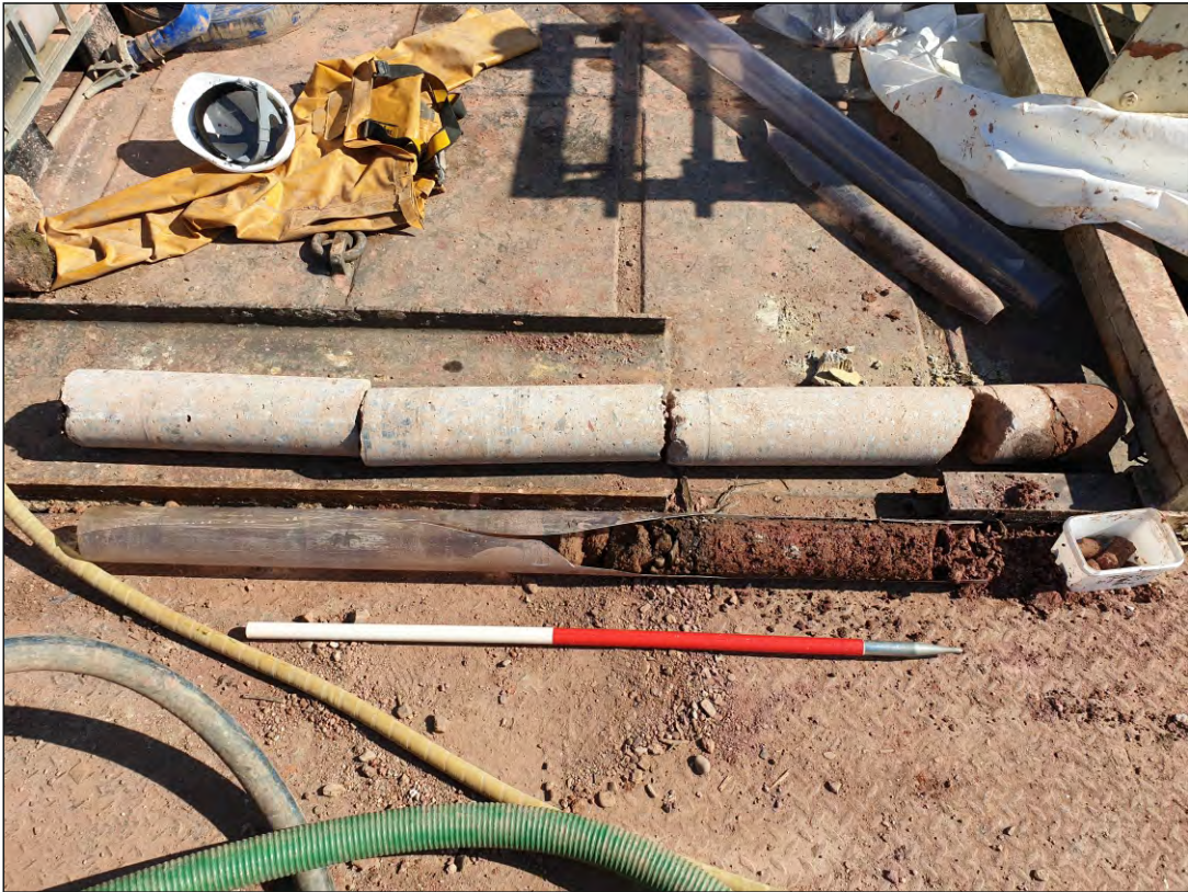
Pl. 9 Borehole 7 showing depth of modern concrete repair overlying weir core. 1m scale.
