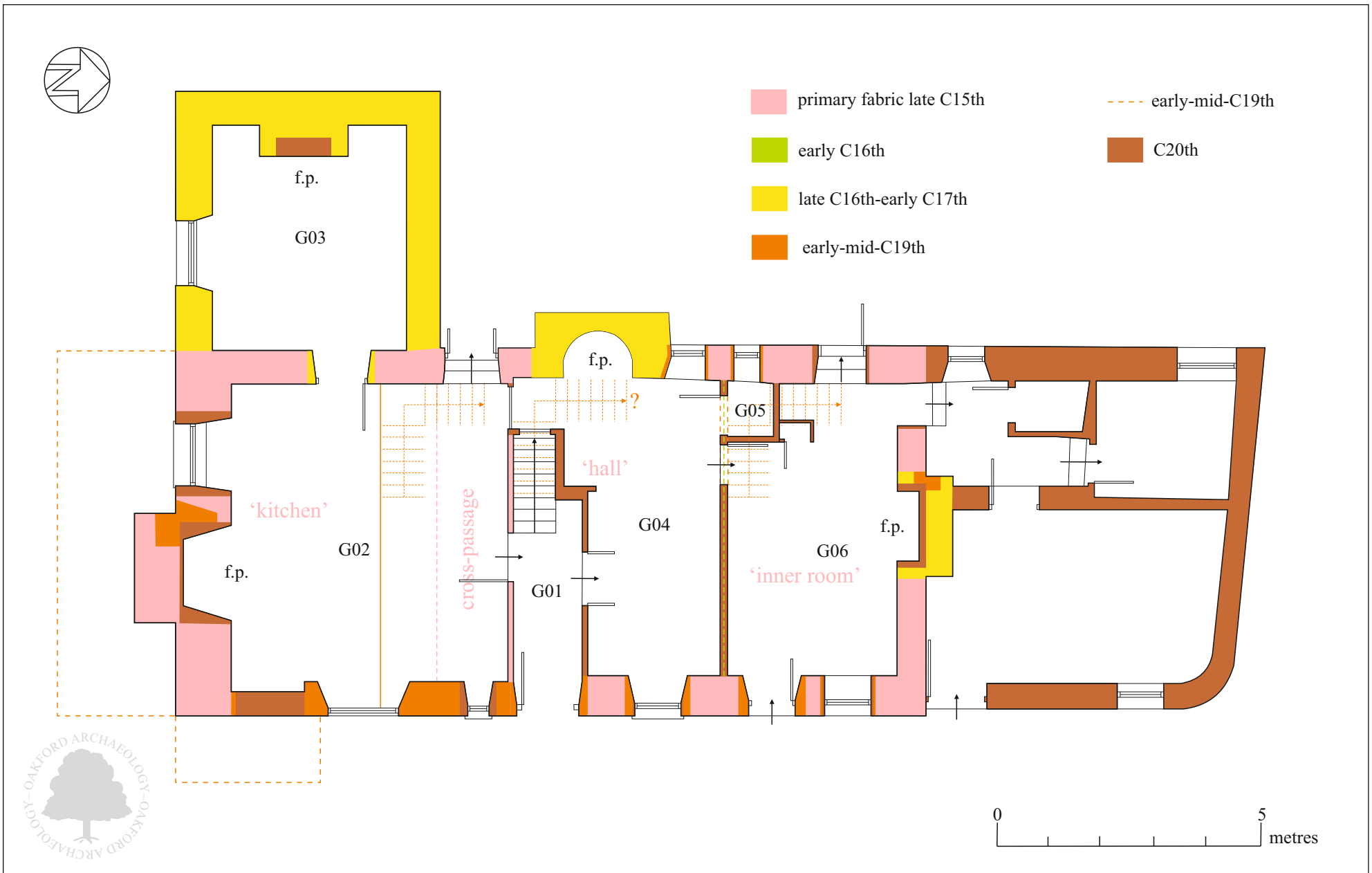
Fig. 6 Plan of ground-floor showing location of observations and suggested phases of development.
