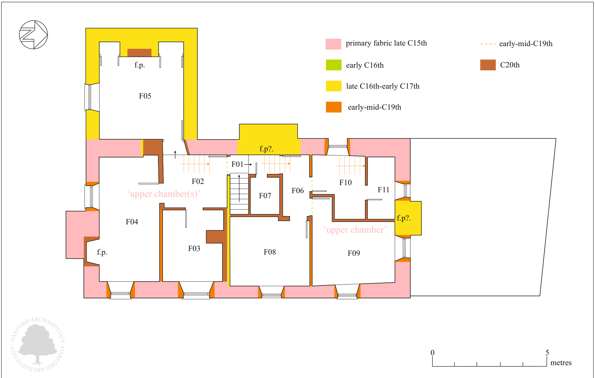
Fig. 8 Plan of the first-floor showing locations of observations and suggested phase of development.
