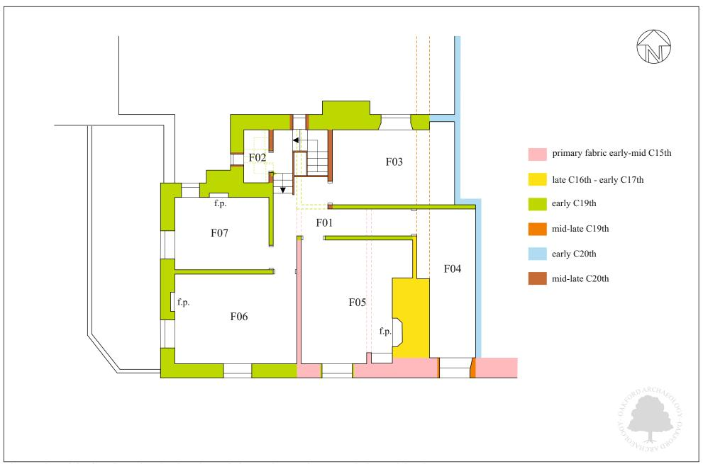
Fig. 14 Plan of the first-floor showing locations of observations and suggested phase of development.
