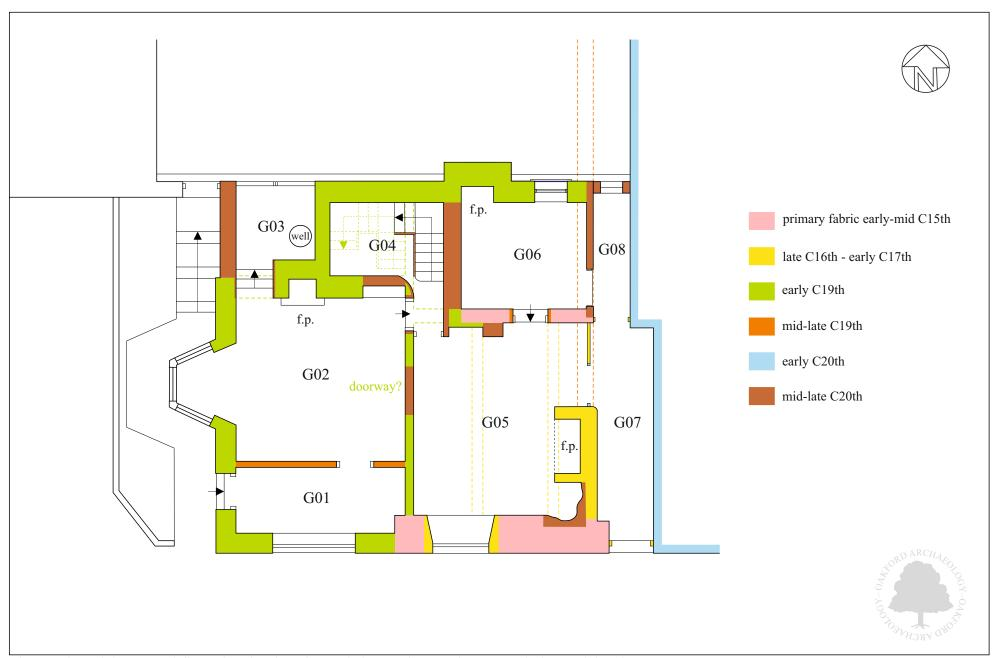
Fig. 13 Plan of the ground-floor showing locations of observations and suggested phase of development.
