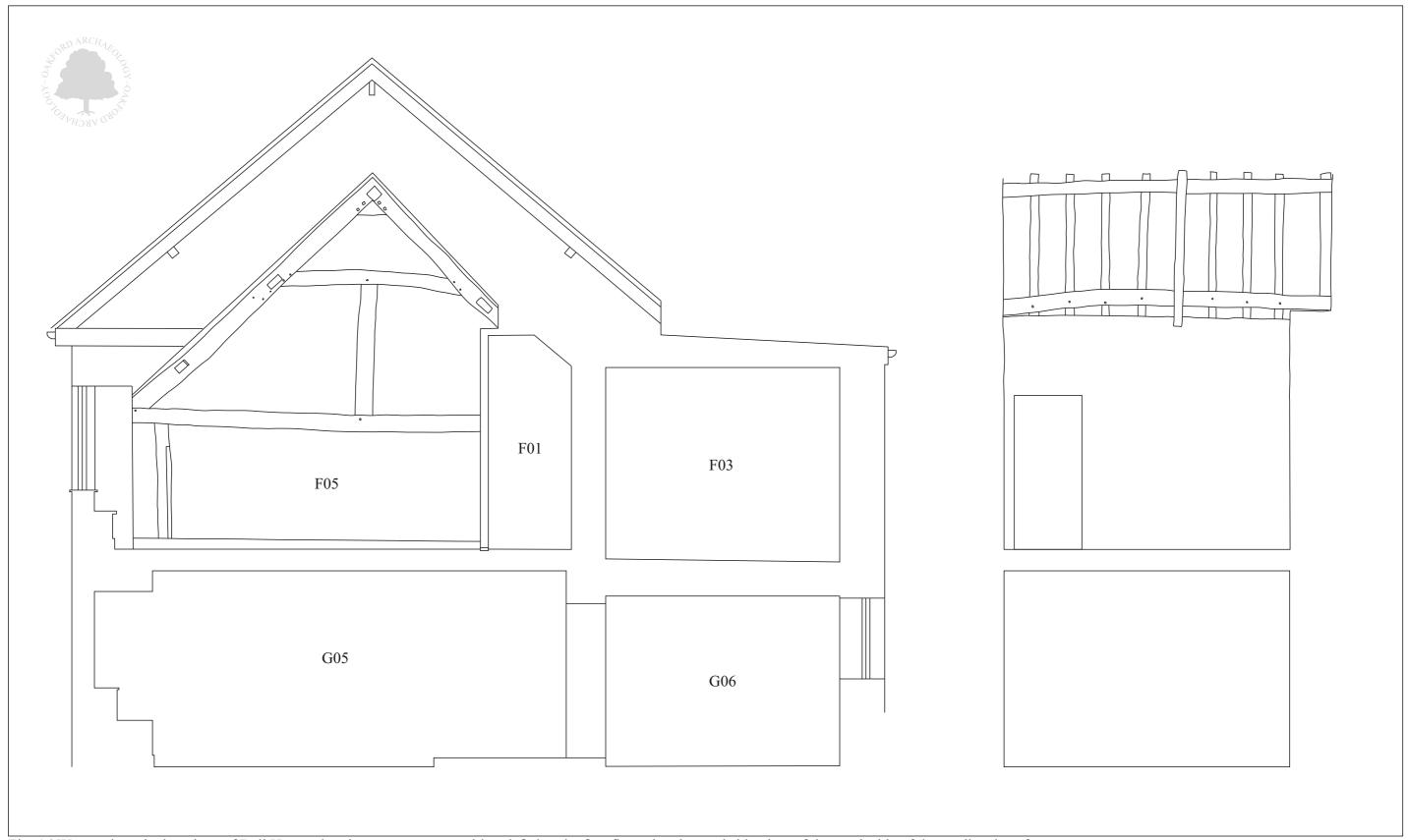
Fig. 16 West and north elevations of Bell House showing crown strut partition defining the first floor chamber and side view of the north side of the medieval roof.
