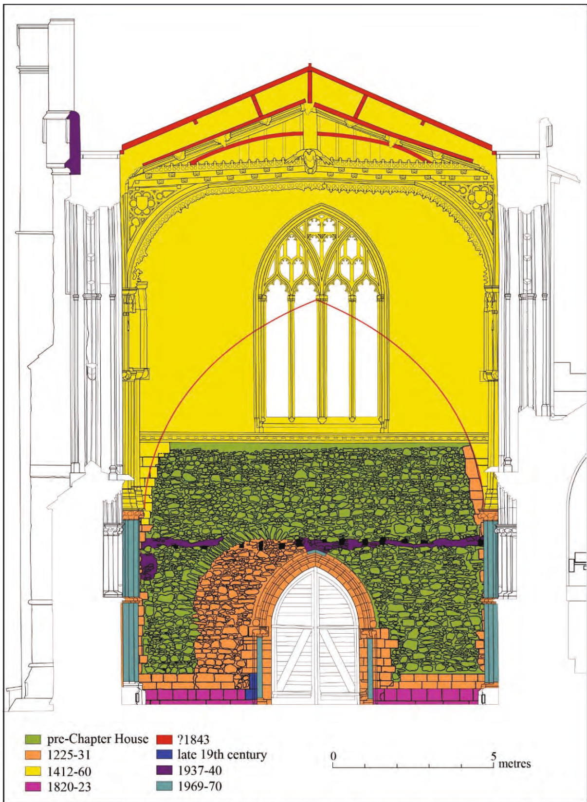
Fig. 4c. The Chapter House, internal face of the west wall: phasing with reconstruction of primary wooden vault ( J. Allan & J. Sampson 1996, with corrections/additions, J. Allan 2020 and 2021 ).
