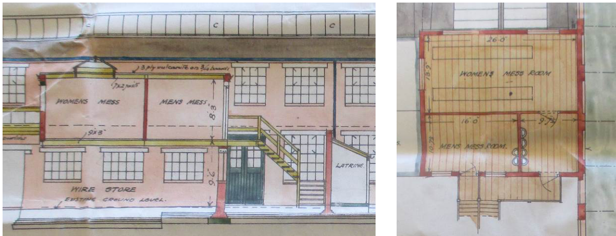
Cross-section (left) and first floor plan (right) of Bldg. 13e; extracted for original design drawings (BBP 31880, 1920).
