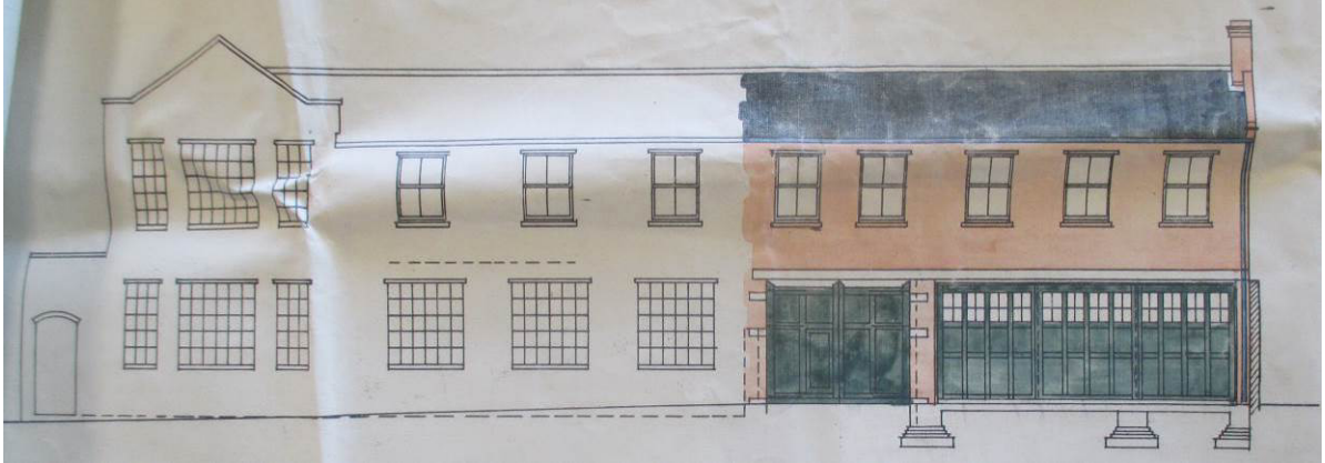
Building 13 , as extended 1920 (BBP 31180 ); north elevation to Northwood Street, extended by five window bays ( 13c ).
