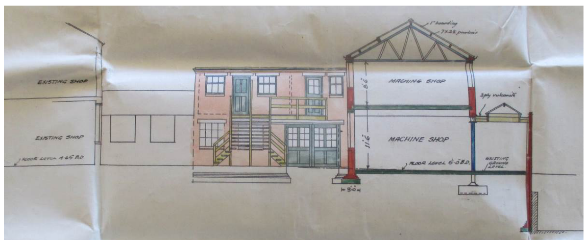
Bldg. 13 , as extended 1920 (BBP 31180 ); cross-sectional elevation through site looking south; cross-section of shopping range 13d to right, with wire store/mess room 13e to centre ( NB. external stair access).
