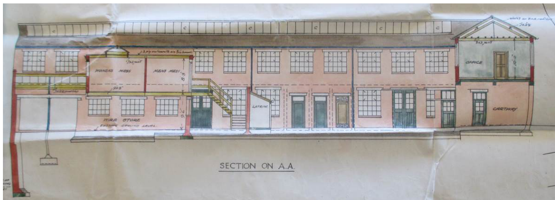
Bldg. 13 , as extended 1920 (BBP 31180 ); cross-sectional elevation through site looking west; east elevation of shopping range 13d , cross-section of 13c to right, and wire store/mess room 13e and covered yard 13f to left.
