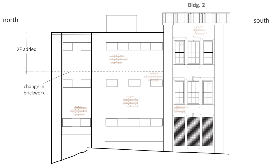
(b) elevation to Newhall Street
