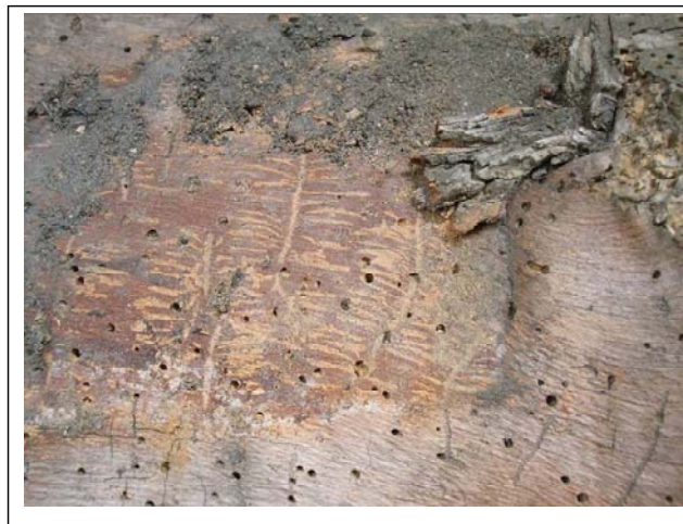
Figure 3: Horizontal worm burrows forming crevices to the surface of the sapwood, just below the bark, are another distinctive feature of elm.
