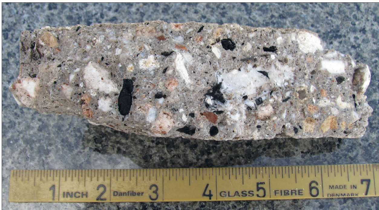
Figure 1 The upper layer of gypsum-plaster and lime-ash with fragments of charcoal, gypsum (white), burnt limestone (grey) and red shale clearly visible. Photo by Peter M. Allen.
